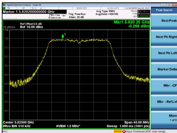
(802.11ac20) PSD plot on channel 165
