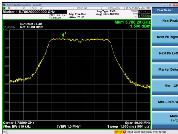
(802.11ac20) PSD plot on channel 165
