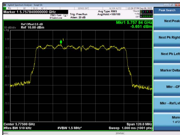
(802.11ac80) PSD plot on channel 155
