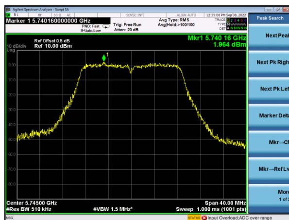
(802.11n20) PSD plot on channel 157
