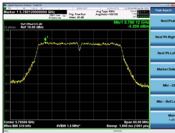
(802.11ac40) PSD plot on channel 159
