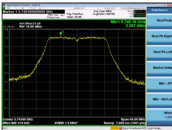
(802.11ac20) PSD plot on channel 157
