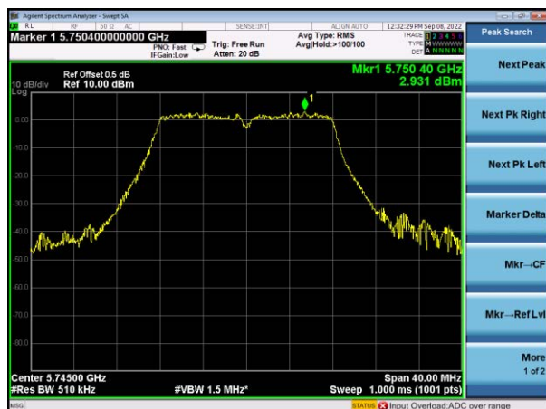
(802.11a) PSD plot on channel 157
