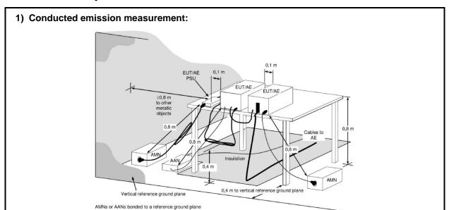
**Note:** The 0.8 m distance specified between EUT/AE/PSU and AMN/AAN, is applicable only to the EUT being measured. If the device is AE then it shall be >0.8 m.
