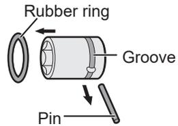
② Insert the socket into the tool.
