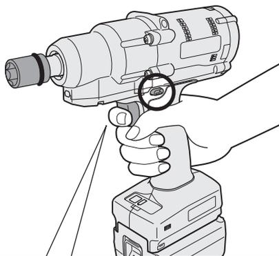
For about 1 second just after a battery pack is attached, trigger switch pull-in operation is not accepted.
