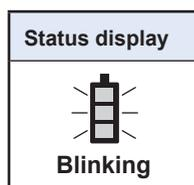
This is a function to shut off power to the tool when battery voltage dropped to a certain standard. When it functions, even if you pull the trigger switch, the tool will not move until you charge the battery pack (or replace it with another battery pack that is charged).
