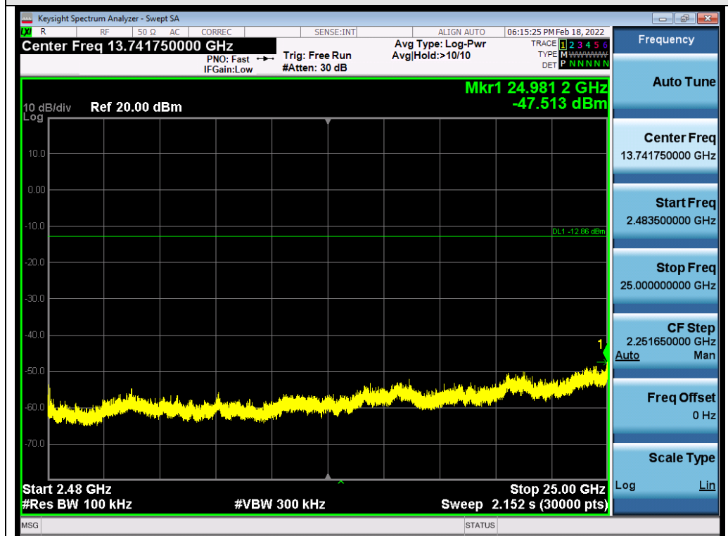
Test_Graph_GFSK_ANT1_2441_Higher Band Emissions
