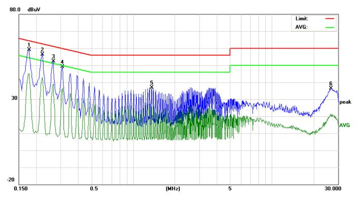
Line Conducted Emission Test Line 1-L
