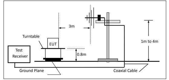
(C) Radiated Emission Test-Up Frequency Above 1GHz
