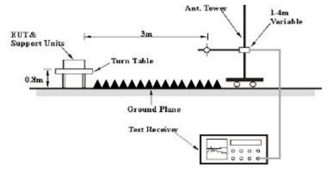
The radiated emission was performed in the 3 meters chamber test site, using the setup accordance with the ANSI C63.4-2014. The specification used was with the FCC Part 15 B Class B limits.
