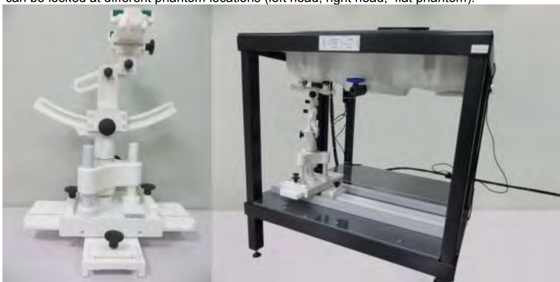
Device holder supplied by SATIMO
