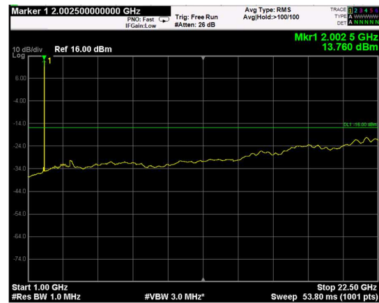
Channel: BOTTOM, Modulation: QPSK, BW=15MHz, Range: Upper
