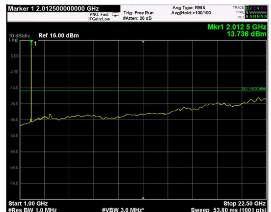
Channel: TOP, Modulation: 256QAM, BW=15MHz, Range: Upper
