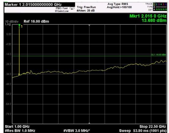
Channel: TOP, Modulation: QPSK, BW=10MHz, Range: Upper
