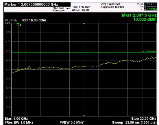
Channel: MIDDLE, Modulation: 256QAM, BW=5MHz, Range: Upper
