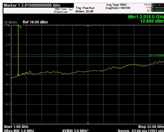
Channel: TOP, Modulation: 256QAM, BW=10MHz, Range: Upper
