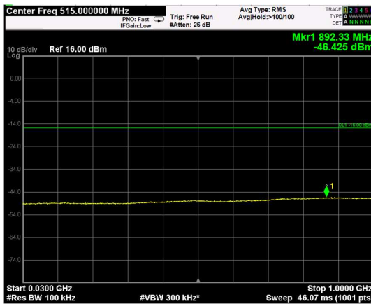
Channel: MIDDLE, Modulation: 256QAM, BW=5MHz, Range: Lower
