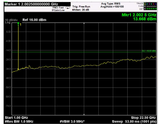
Channel: BOTTOM, Modulation: 64QAM, BW=15MHz, Range: Upper
