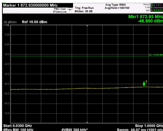
Channel: TOP, Modulation: 16QAM, BW=15MHz, Range: Lower
