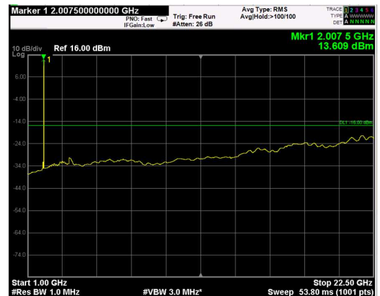
Channel: MIDDLE, Modulation: 64QAM, BW=15MHz, Range: Upper
