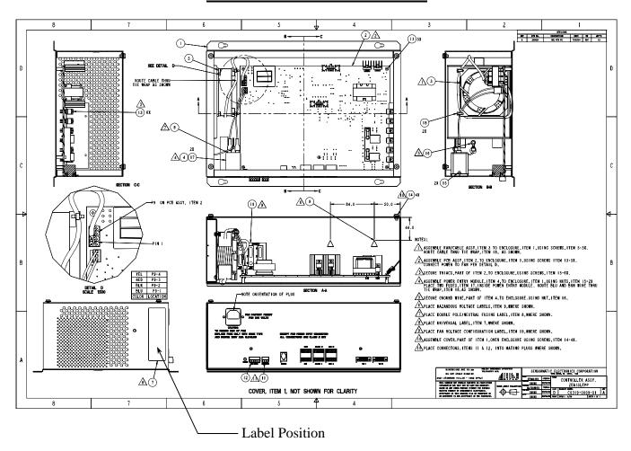
The label is a metalized polyester that is UL recognized and is permanently affixed using an L-23 adhesive.
