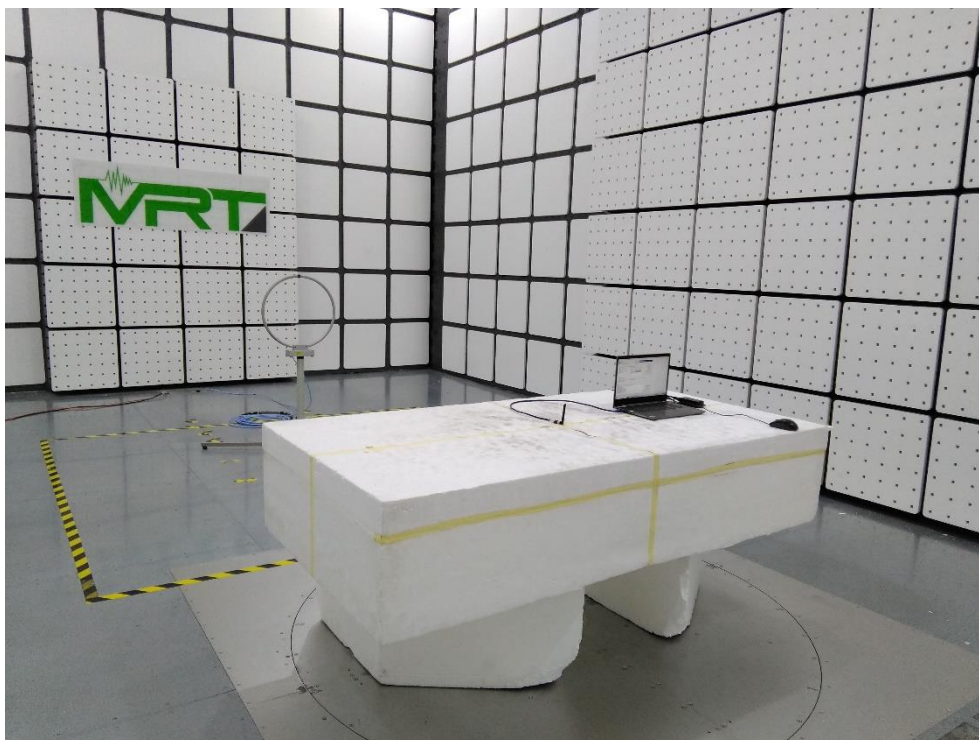
Description: Radiated Emission Test Setup for 9kHz~30MHz
