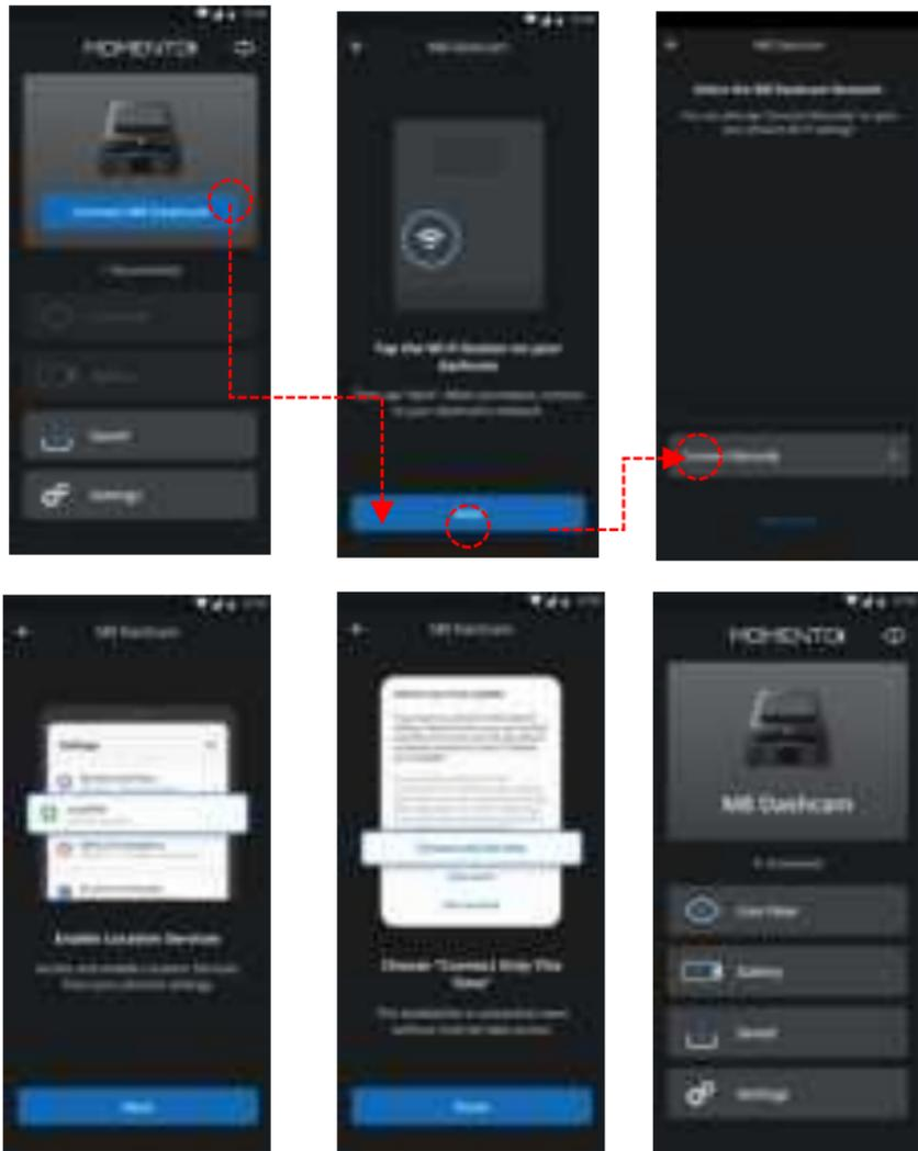
Manual Connect is required for the initial setup. Find the M8's Wi-Fi network on your phone's Wi-Fi network list and connect by using the password "12345678", then return to the App.
