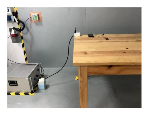
Set-up for Radiated Emission (RE), Below 1GHz
