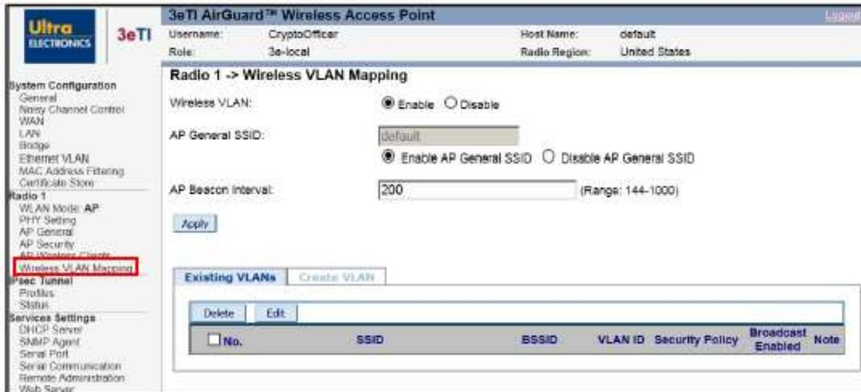
Figure 48: Radio – Wireless VLAN Mapping – Enable Wireless VLAN
