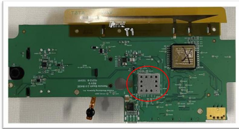
With Shield Can Installed (Bottom)
