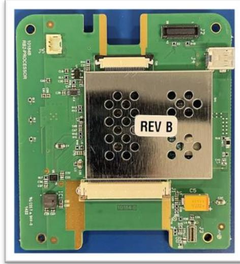
With Shield Can Installed
