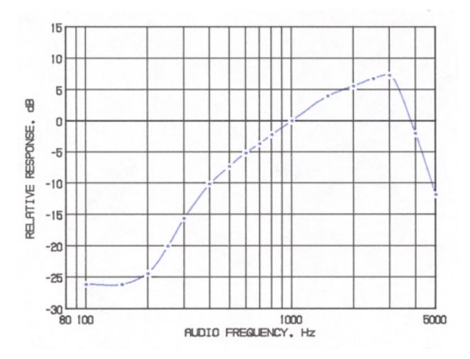
MODULATION FREQUENCY RESPONSE FCC ID: MMAFG2
