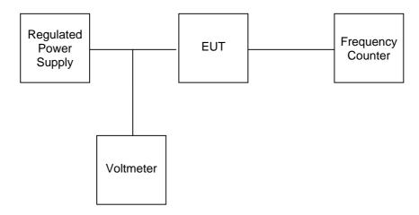
2. For battery powered equipment, reduce primary supply voltage to the battery operating end point voltage which is specified by the manufacturer.
