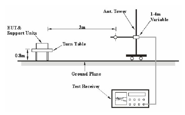
The radiated emission tests were performed in the 3 meters chamber A test site, using the setup accordance with the FCC MP - 5. The specification used was the FCC part 18.
