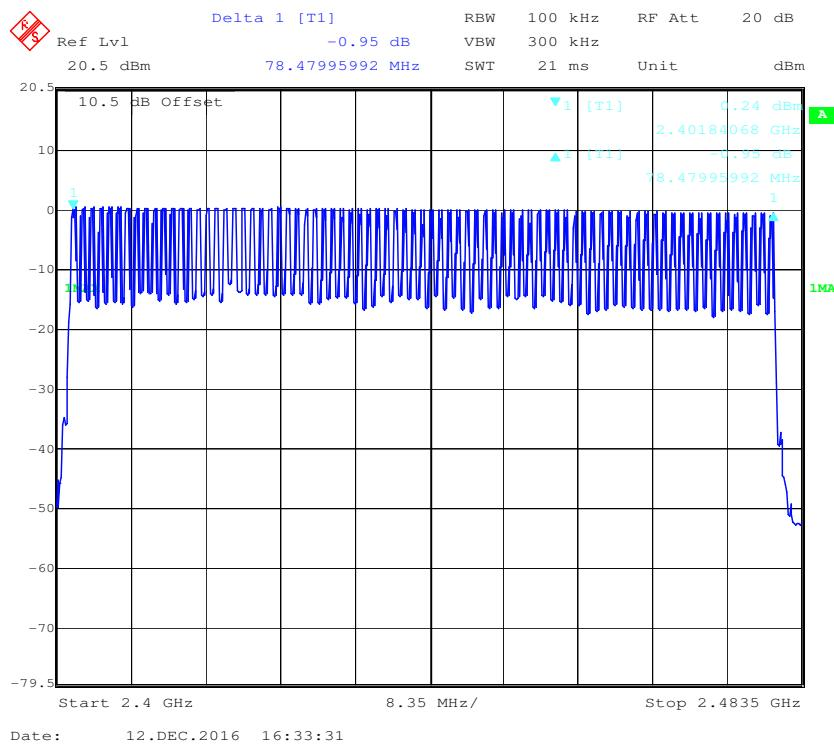
**EDR ( $\pi/4$ -DQPSK): Number of Hopping Channels**
