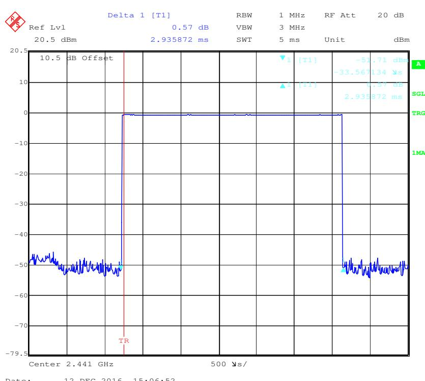
**Pulse time, High Channel, DH5**
