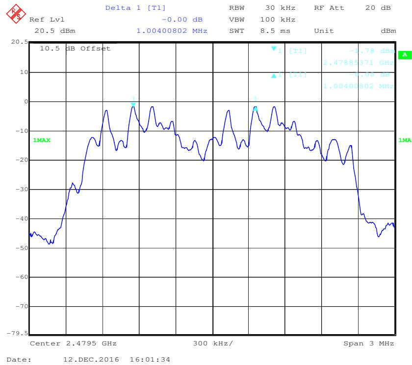
**EDR (8DPSK): Low Channel**
