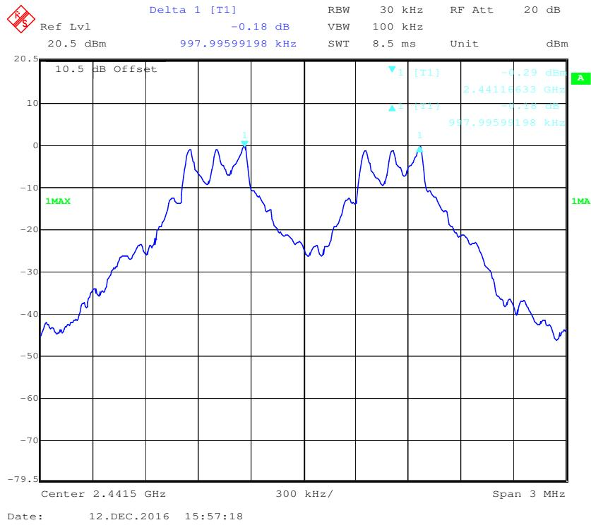
**BDR (GFSK): High Channel**
