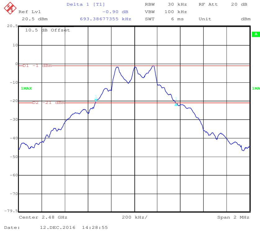
**EDR ( $\pi/4$ -DQPSK): Low Channel**
