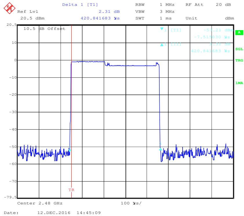
**Pulse time, Low Channel, 2DH3**
