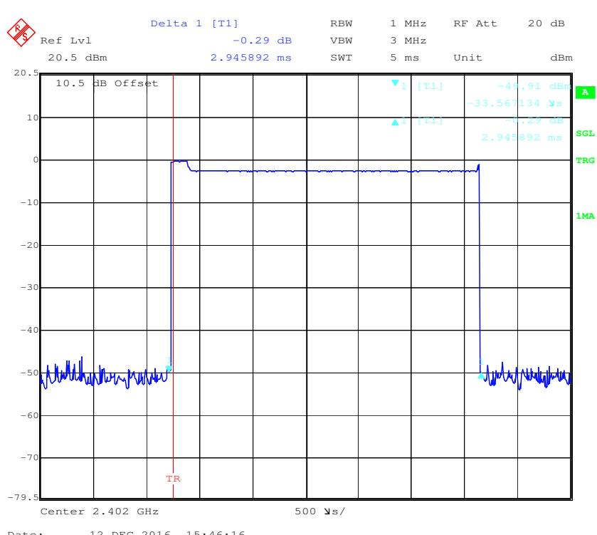
**Pulse time, Middle Channel, 2DH5**
