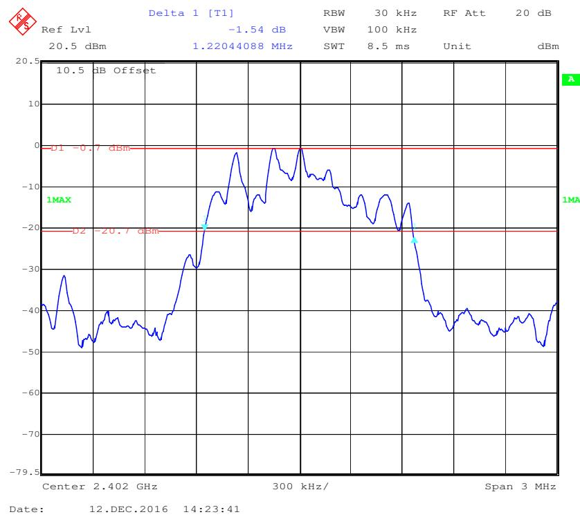
**EDR ( $\pi/4$ -DQPSK): Middle Channel**
