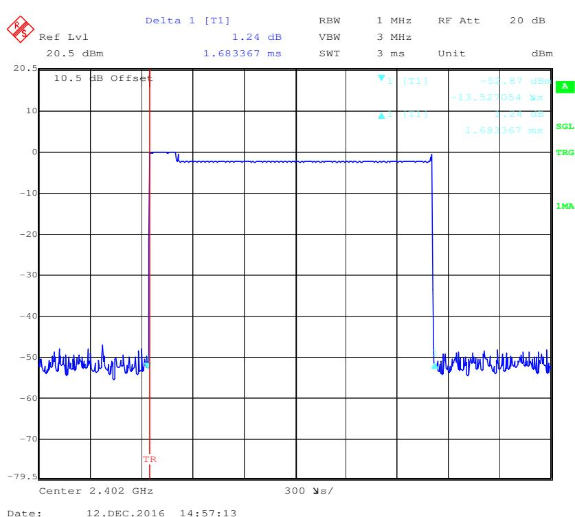
**Pulse time, Middle Channel, 3DH3**
