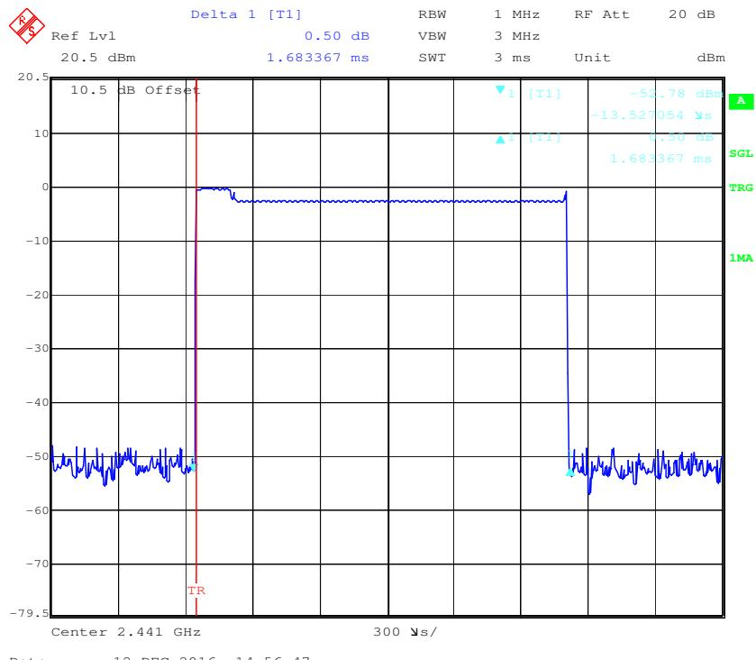
**Pulse time, High Channel, 3DH3**
