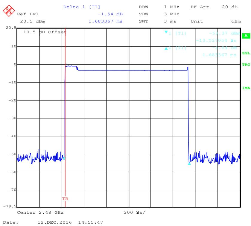
**Pulse time, Low Channel, 3DH5**
