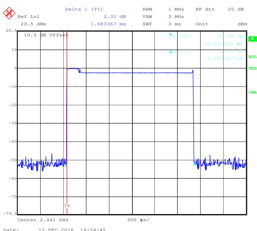
**Pulse time, High Channel, 2DH3**
