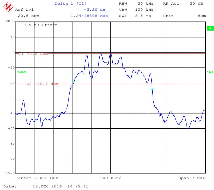
**EDR (8DPSK): Middle Channel**
