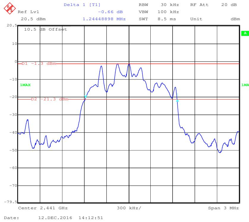
**EDR (8DPSK): High Channel**
