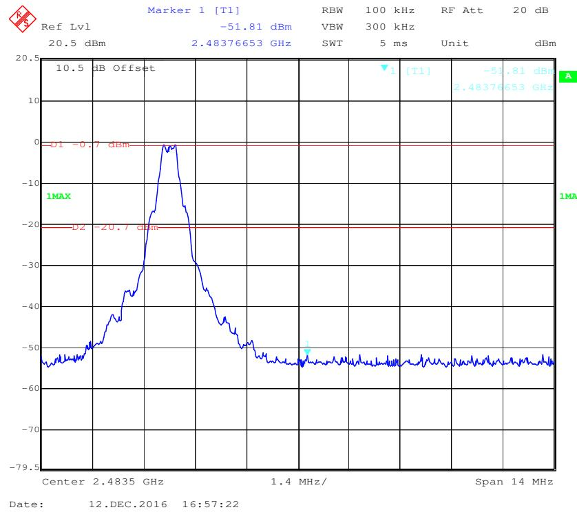
**EDR ( $\pi/4$ -DQPSK): Band Edge-Left Side**
