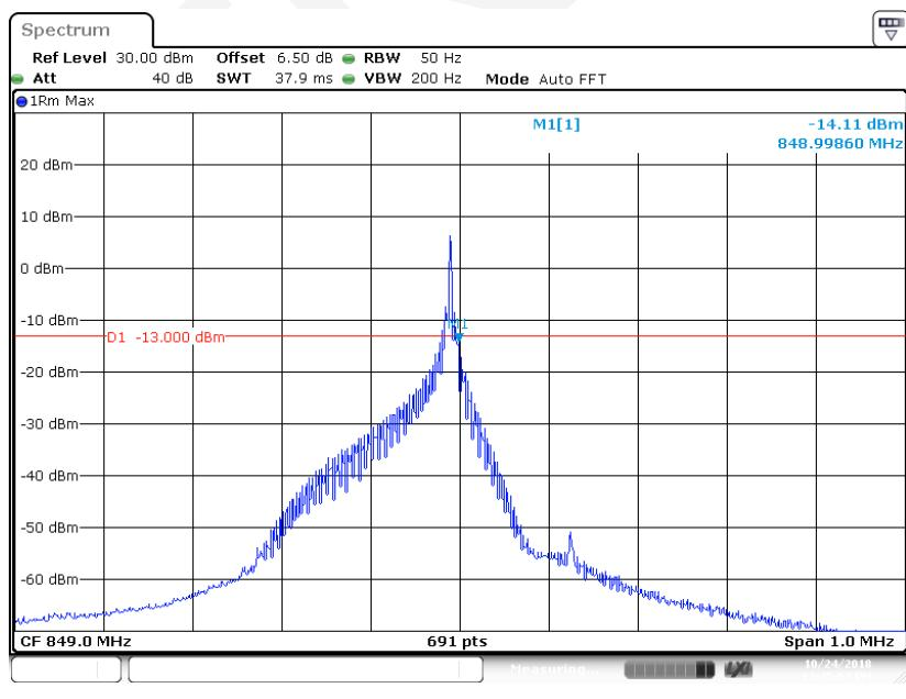
**BPSK (15kHz, 1#0) - Left Band Edge**
