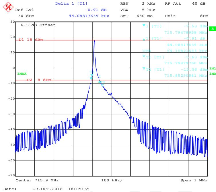
**BPSK (15kHz,1#0) - 99% Occupied & 26 dB Emissions Bandwidth, High channel**
