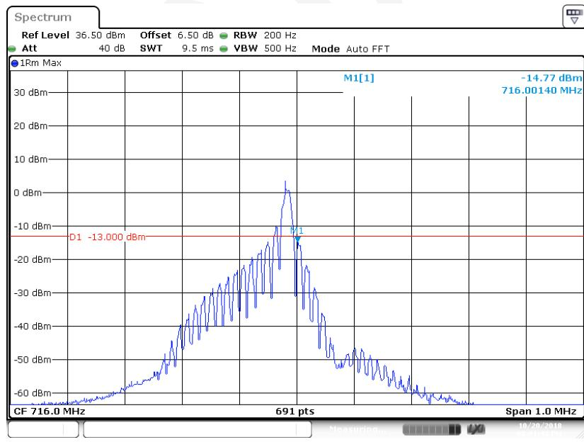
**QPSK (3.75kHz, 1#0) - Left Band Edge**
