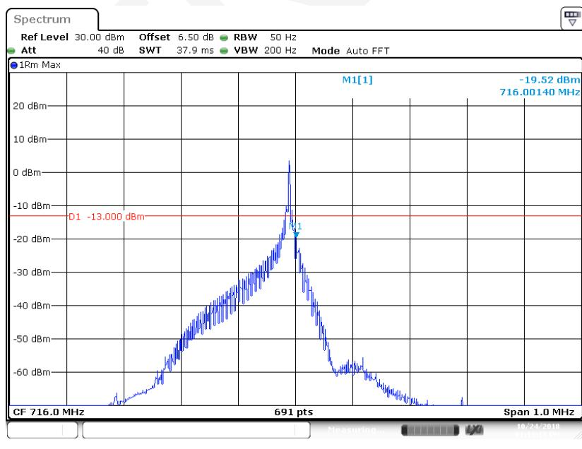
**BPSK (15kHz, 1#0) - Left Band Edge**
