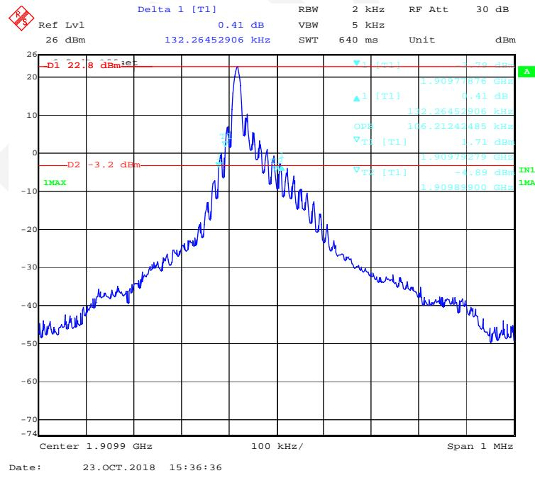
**QPSK (15kHz,12#0) - 99% Occupied & 26 dB Emissions Bandwidth, High channel**
