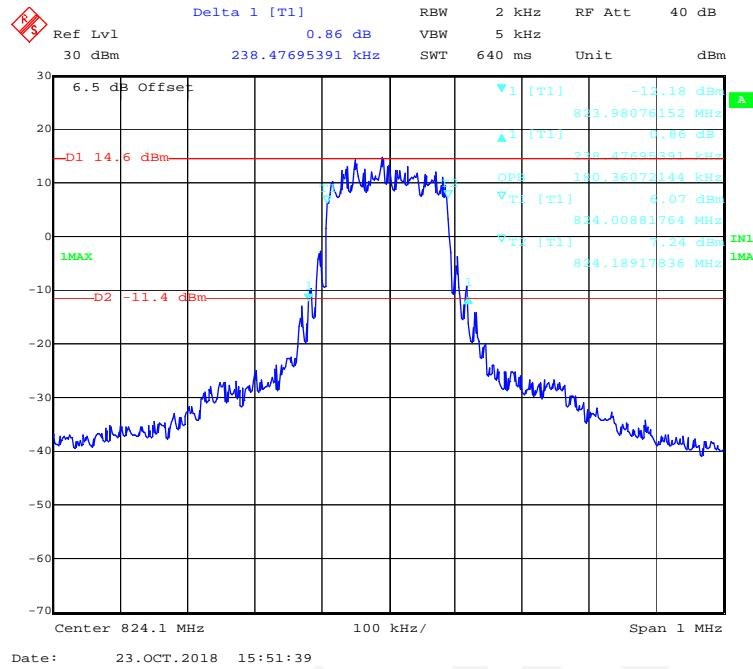
**QPSK (3.75kHz,1#0) - 99% Occupied & 26 dB Emissions Bandwidth, Middle channel**
