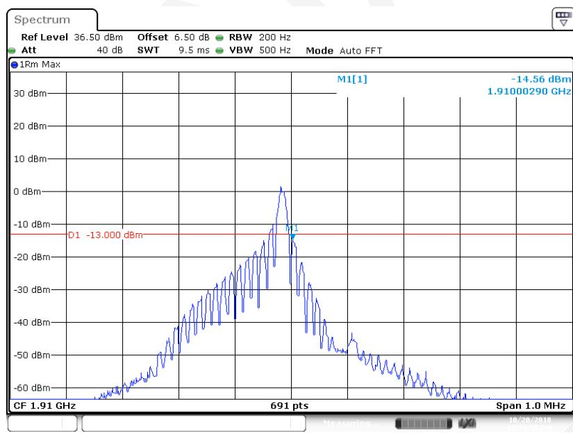
**QPSK (3.75kHz, 1#0) - Left Band Edge**
