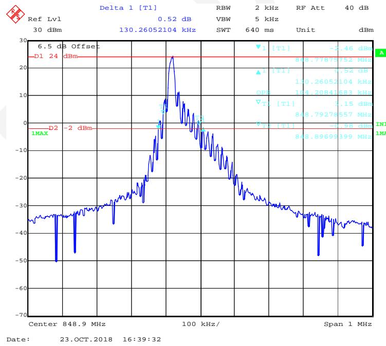
**QPSK (15kHz,12#0) - 99% Occupied & 26 dB Emissions Bandwidth, High channel**
