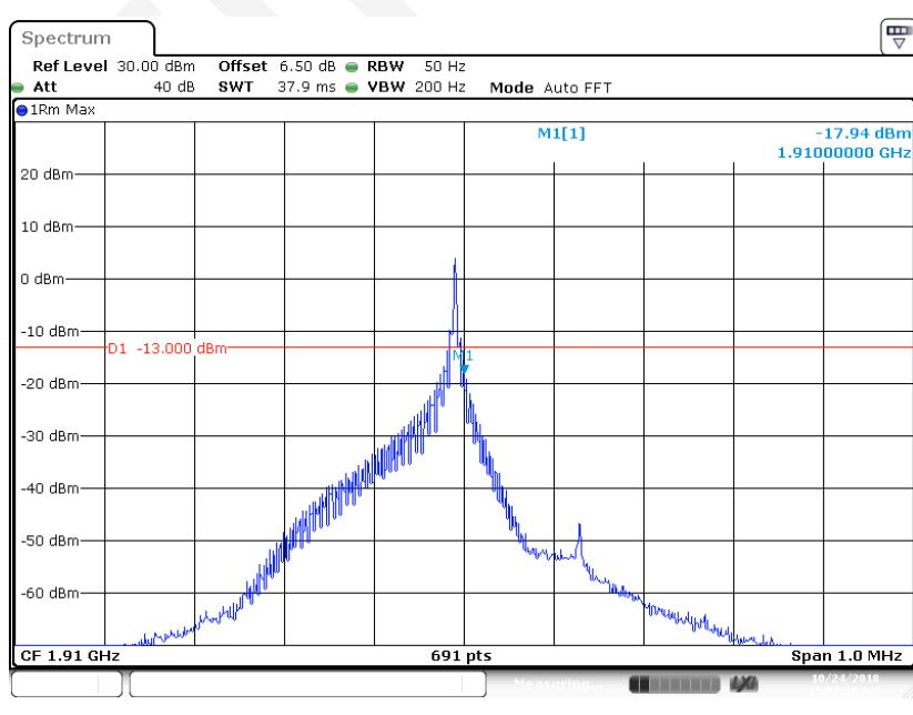
**BPSK (15kHz, 1#0) - Left Band Edge**
