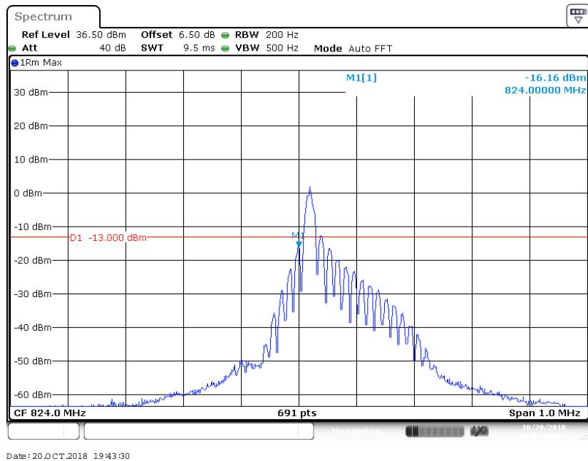
**QPSK (15kHz, 1#11) - Right Band Edge**
