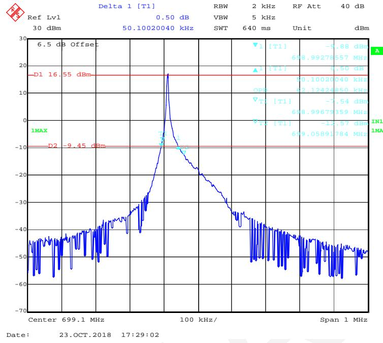
**QPSK (15kHz,1#0) - 99% Occupied & 26 dB Emissions Bandwidth, Low channel**
