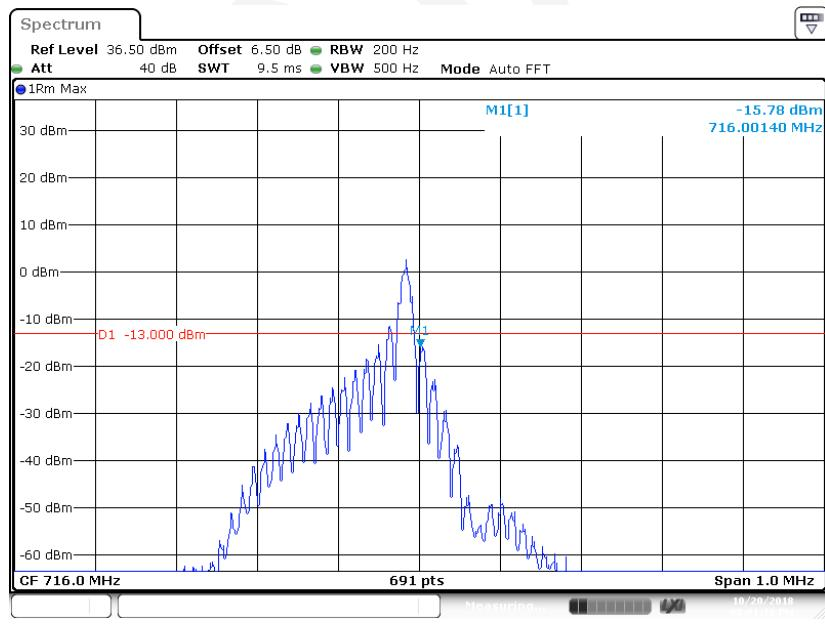
**QPSK (15kHz, 12#0) - Left Band Edge**
