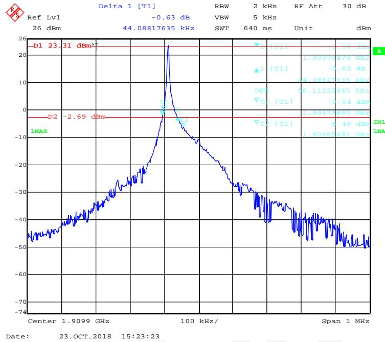
**BPSK (15kHz,1#0) - 99% Occupied & 26 dB Emissions Bandwidth, High channel**
