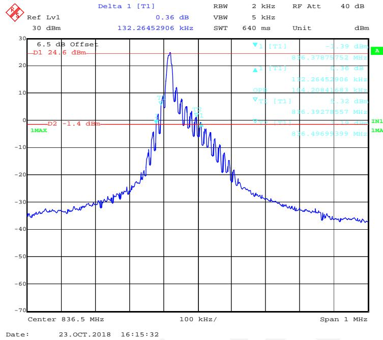
**QPSK (15kHz,12#0) - 99% Occupied & 26 dB Emissions Bandwidth, Middle channel**
