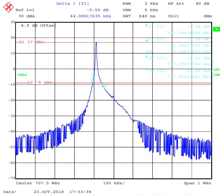
**BPSK (15kHz,1#0) - 99% Occupied & 26 dB Emissions Bandwidth, Middle channel**
