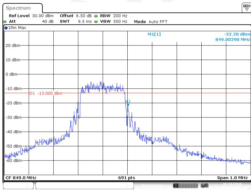
**NB-IoT Band 12:****BPSK (3.75kHz, 1#0) - Left Band Edge**
