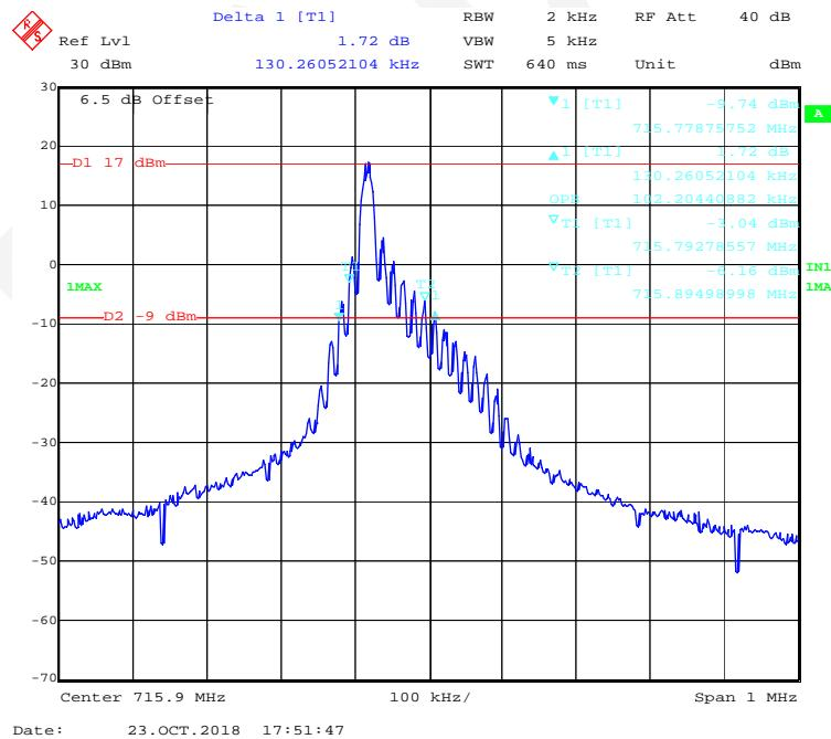
**QPSK (15kHz,12#0) - 99% Occupied & 26 dB Emissions Bandwidth, High channel**
