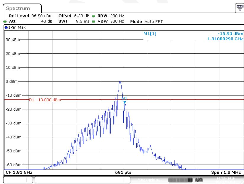
**QPSK (15kHz, 12#0) - Left Band Edge**
