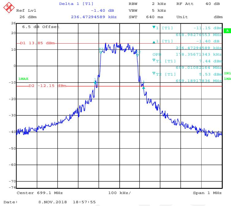
**QPSK (3.75kHz,1#0) - 99% Occupied & 26 dB Emissions Bandwidth, Middle channel**
