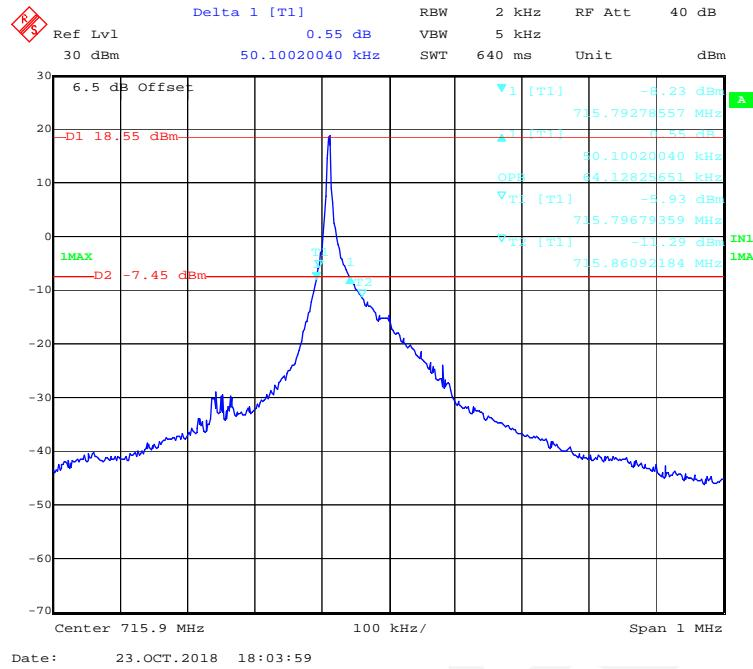
**QPSK (15kHz,1#0) - 99% Occupied & 26 dB Emissions Bandwidth, High channel**
