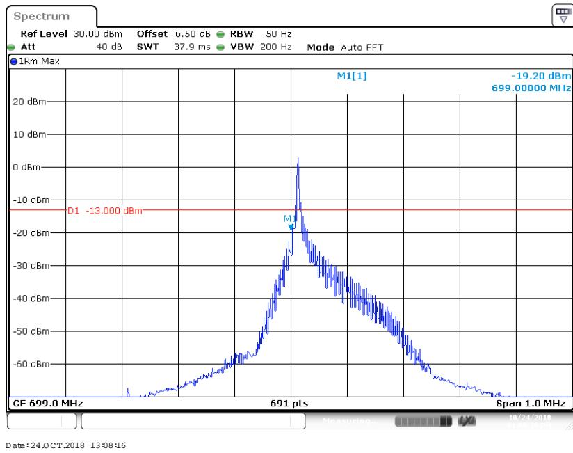
**QPSK (3.75kHz, 1#47) - Right Band Edge**
