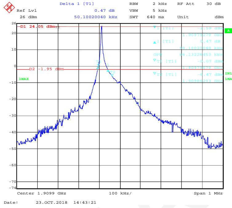
**QPSK (15kHz,1#0) - 99% Occupied & 26 dB Emissions Bandwidth, High channel**
