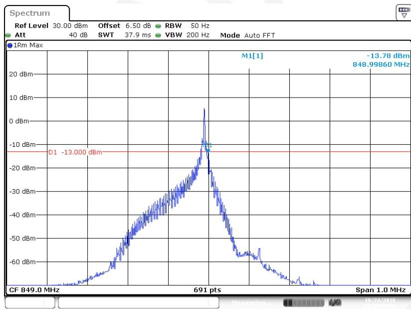
**QPSK (15kHz, 1#0) - Left Band Edge**
