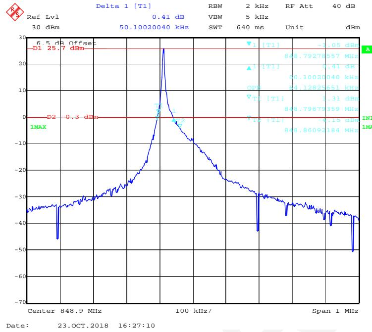
**QPSK (15kHz,1#0) - 99% Occupied & 26 dB Emissions Bandwidth, High channel**
