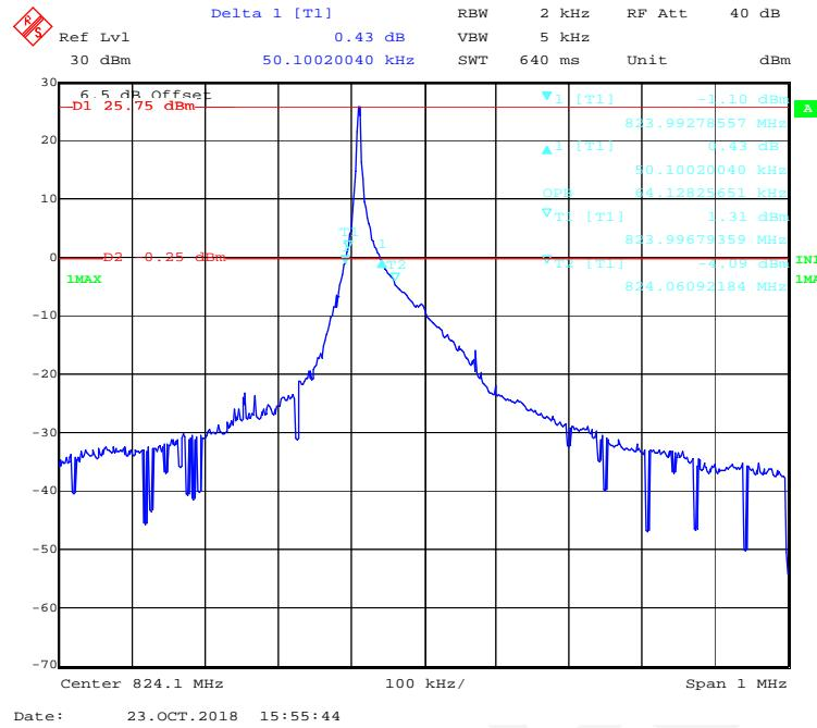
**QPSK (15kHz,1#0) - 99% Occupied & 26 dB Emissions Bandwidth, Low channel**
