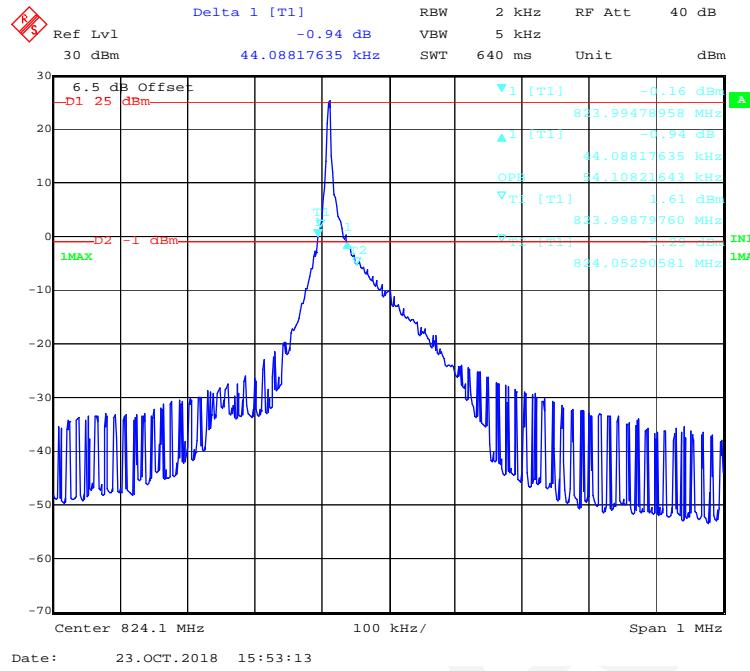
**BPSK (15kHz,1#0) - 99% Occupied & 26 dB Emissions Bandwidth, Low channel**
