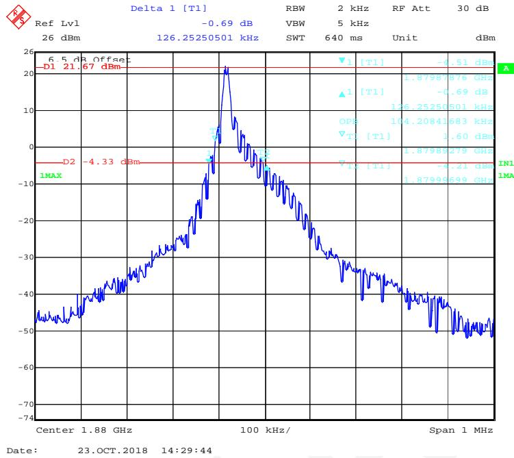
**QPSK (15kHz,12#0) - 99% Occupied & 26 dB Emissions Bandwidth, Middle channel**
