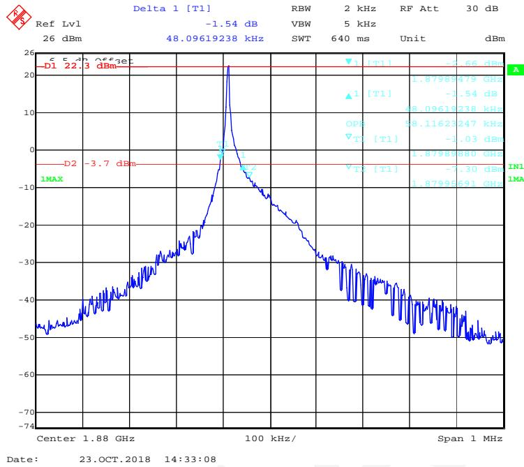
**BPSK (15kHz,1#0) - 99% Occupied & 26 dB Emissions Bandwidth, Middle channel**
