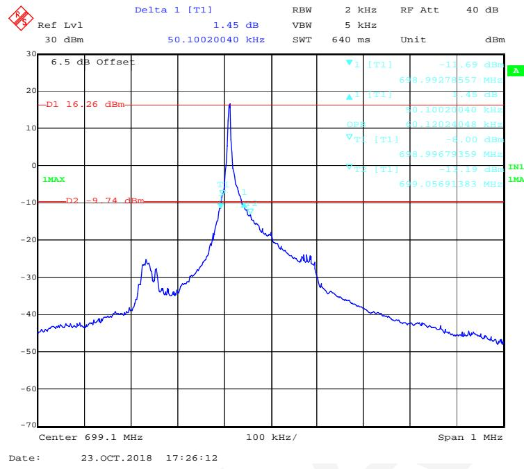
**BPSK (15kHz,1#0) - 99% Occupied & 26 dB Emissions Bandwidth, Low channel**
