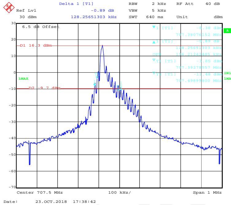
**QPSK (15kHz,12#0) - 99% Occupied & 26 dB Emissions Bandwidth, Middle channel**
