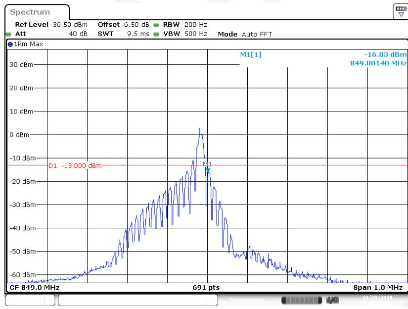
**QPSK (3.75kHz, 1#0) - Left Band Edge**
