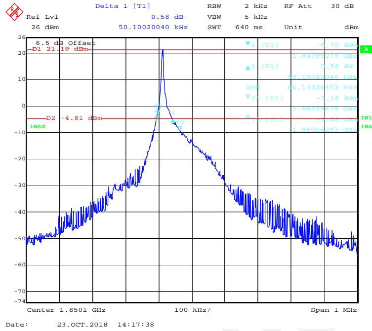
**QPSK (15kHz,1#0) - 99% Occupied & 26 dB Emissions Bandwidth, Low channel**
