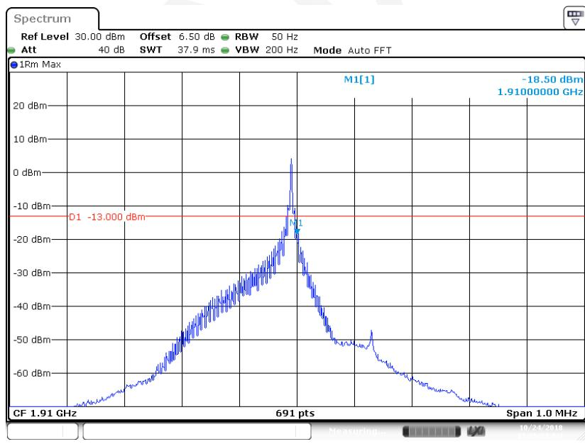
**QPSK (15kHz, 1#0) - Left Band Edge**
