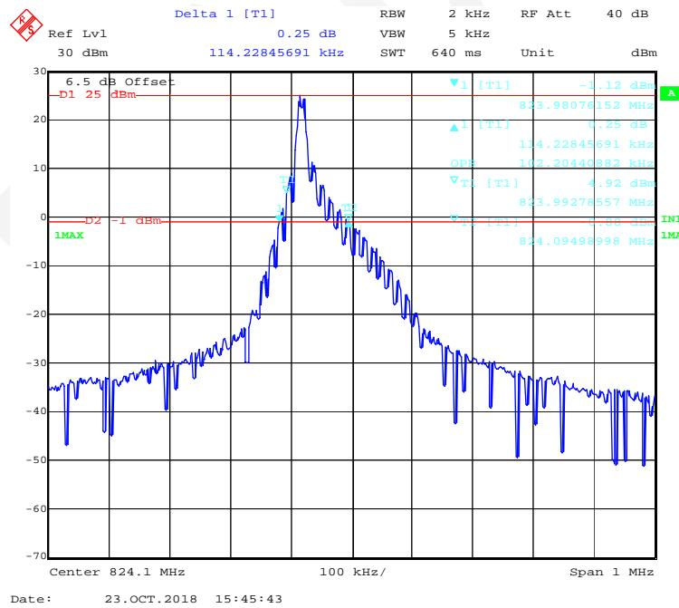
**BPSK (3.75kHz,1#0) - 99% Occupied & 26 dB Emissions Bandwidth, Middle channel**
