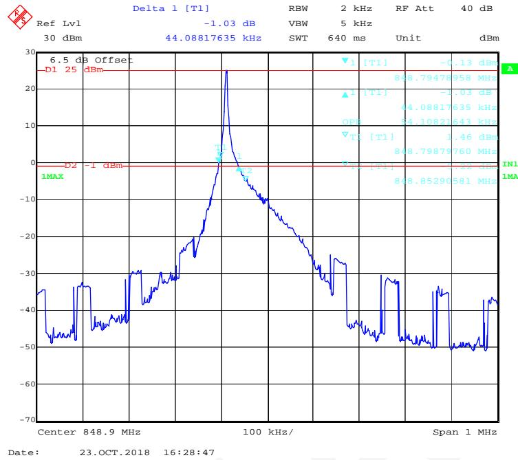
**BPSK (15kHz,1#0) - 99% Occupied & 26 dB Emissions Bandwidth, High channel**
