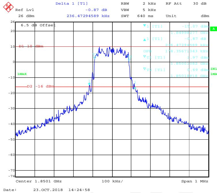
**QPSK (3.75kHz,1#0) - 99% Occupied & 26 dB Emissions Bandwidth, Middle channel**
