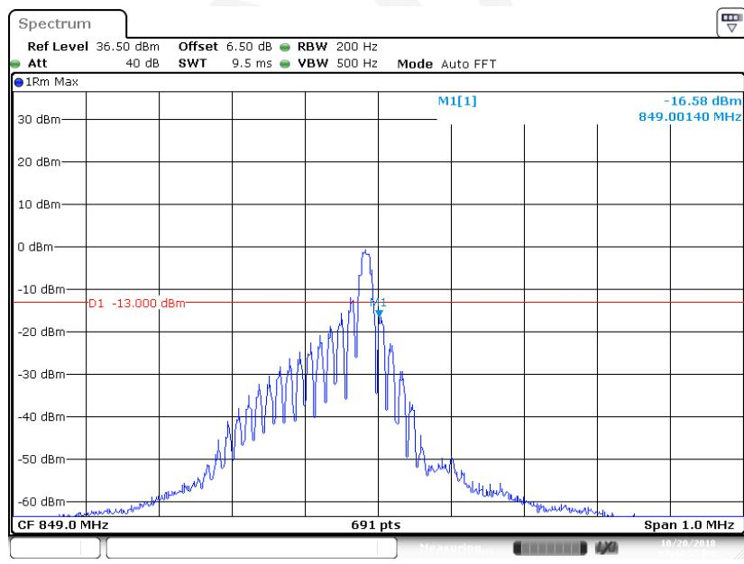
**QPSK (15kHz, 12#0) - Left Band Edge**
