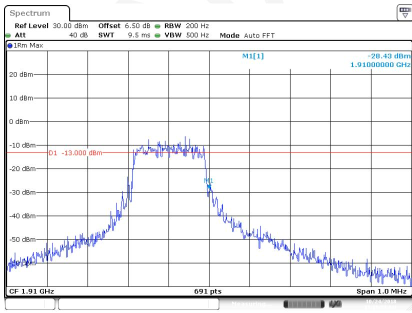
**NB-IoT Band 5:****BPSK (3.75kHz, 1#0) - Left Band Edge**
