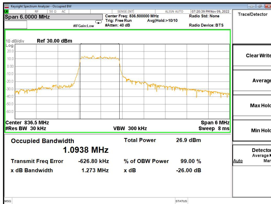
Band26-99% OBW-26915 Channel-3MHz Bandwidth-QPSK
