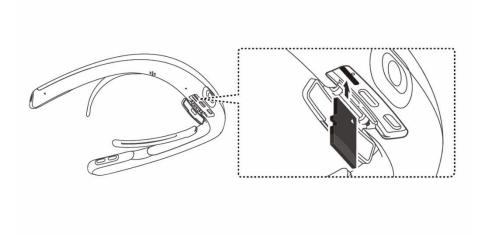
The FITT360 includes 64GB of internal memory. The user can expand storage capacity by installing a memory card of up to 128G.
