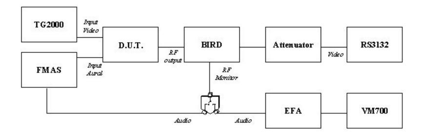
D.U.T. = Device Under Test
