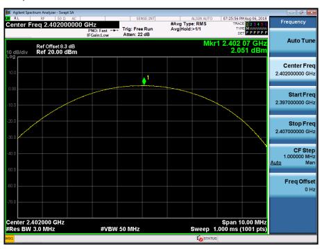
Test Plots (π/4DQPSK) Peak Power (CH.39)
