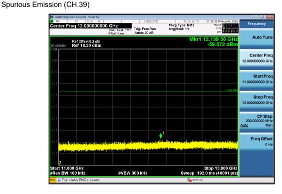
Test Plots (8DPSK)- 13 GHz – 15 GHz Spurious Emission (CH.39)
