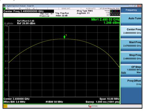
Test Plots (8DPSK) Peak Power (CH.0)
