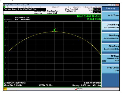
Test Plots (8DPSK) Peak Power (CH.78)
