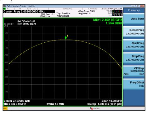
Test Plots (GFSK) Peak Power (CH.39)
