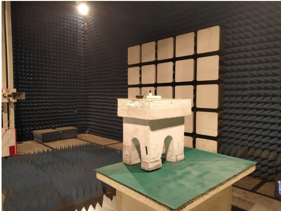
Photograph 3: Set-up for Radiated Spurious Emission, above 1GHz
