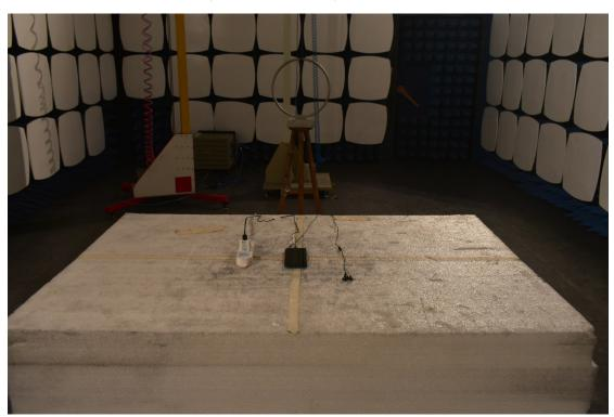
3. Radiated emission (9KHz-30MHz)
