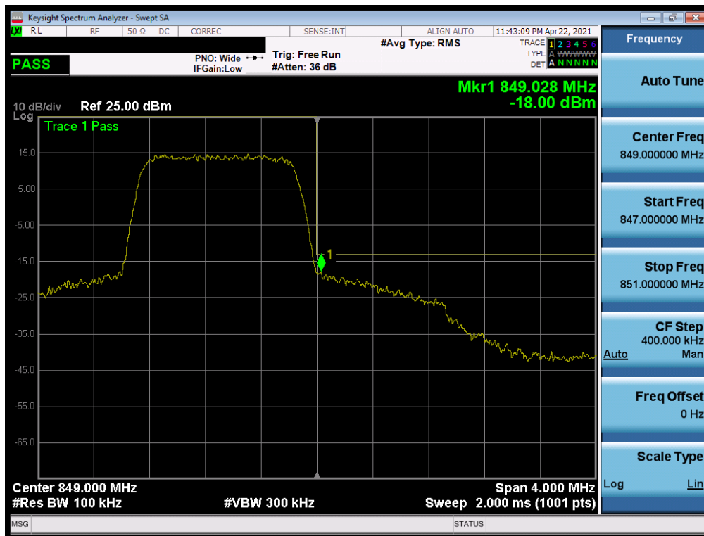
Plot 7-81. Upper Band Edge Plot (LTE Band 26/5 - 1.4MHz QPSK - Full RB)
