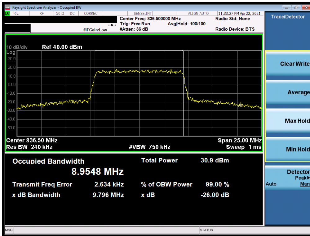
Plot 7-3. Occupied Bandwidth Plot (LTE Band 26/5 10MHz QPSK Full RB)
