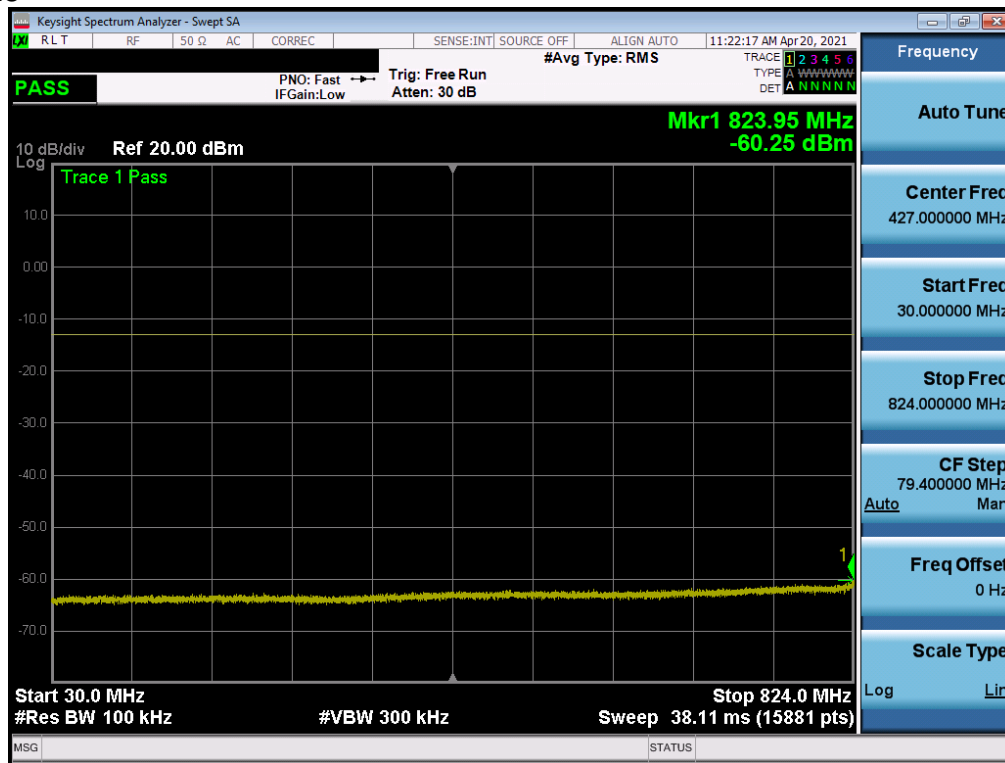
Plot 7-36. Conducted Spurious Plot (NR Band n5 20.0MHz 1 RB Low Channel)
