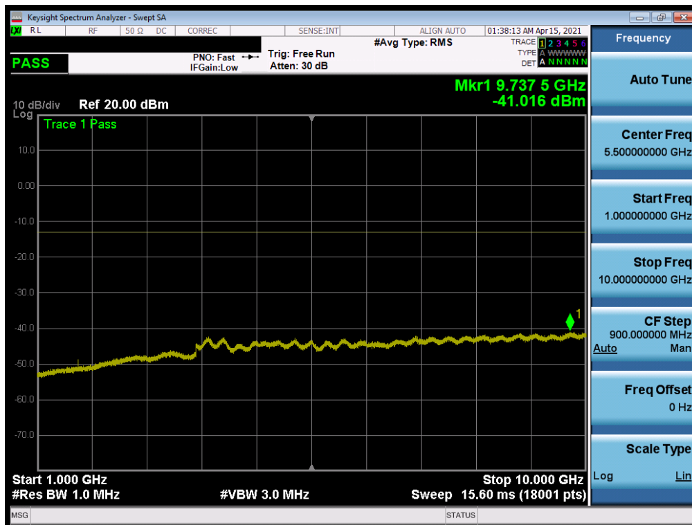
Plot 7-68. Conducted Spurious Plot (CDMA Ch. 384)
