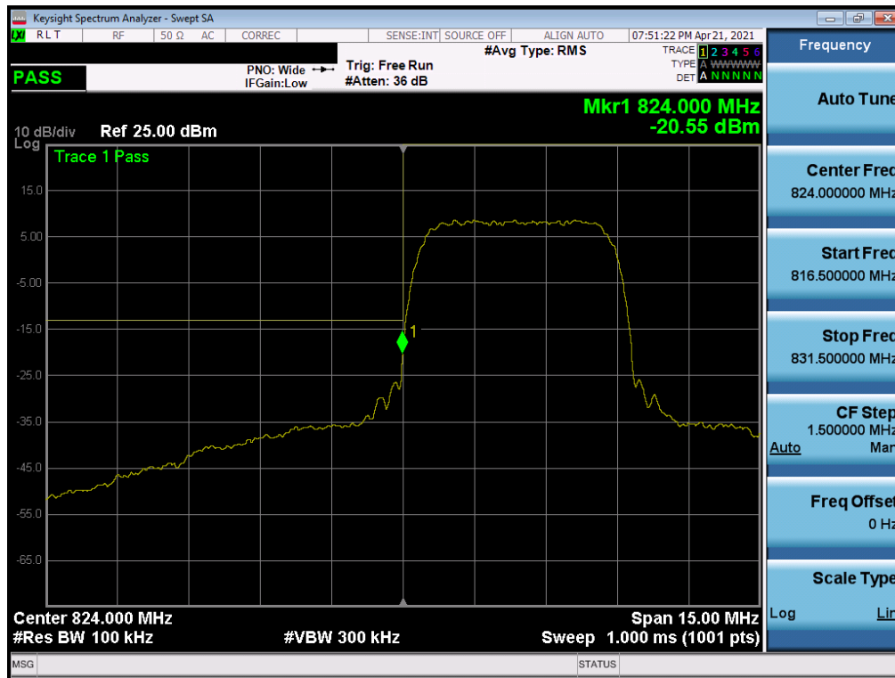
Plot 7-92. Lower Band Edge Plot (WCDMA Cell – Ch. 4132)
