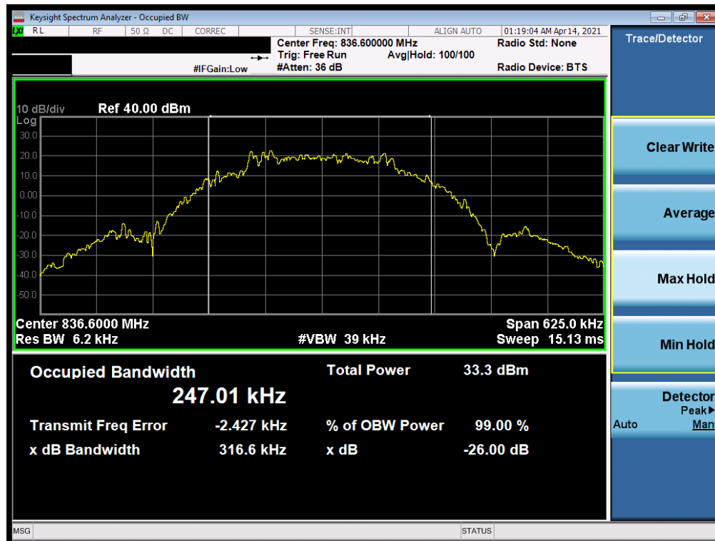
Plot 7-24. Occupied Bandwidth Plot (EDGE, Ch. 190)
