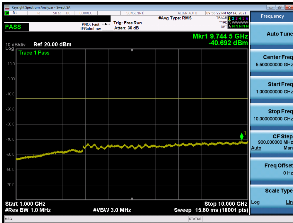
Plot 7-59. Conducted Spurious Plot (WCDMA Ch. 4183)
