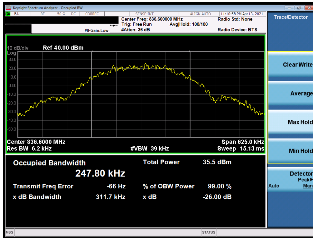
Plot 7-23. Occupied Bandwidth Plot (GPRS, Ch. 190)
