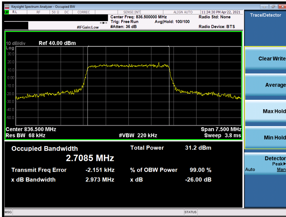
Plot 7-7. Occupied Bandwidth Plot (LTE Band 26/5 3MHz QPSK Full RB)
