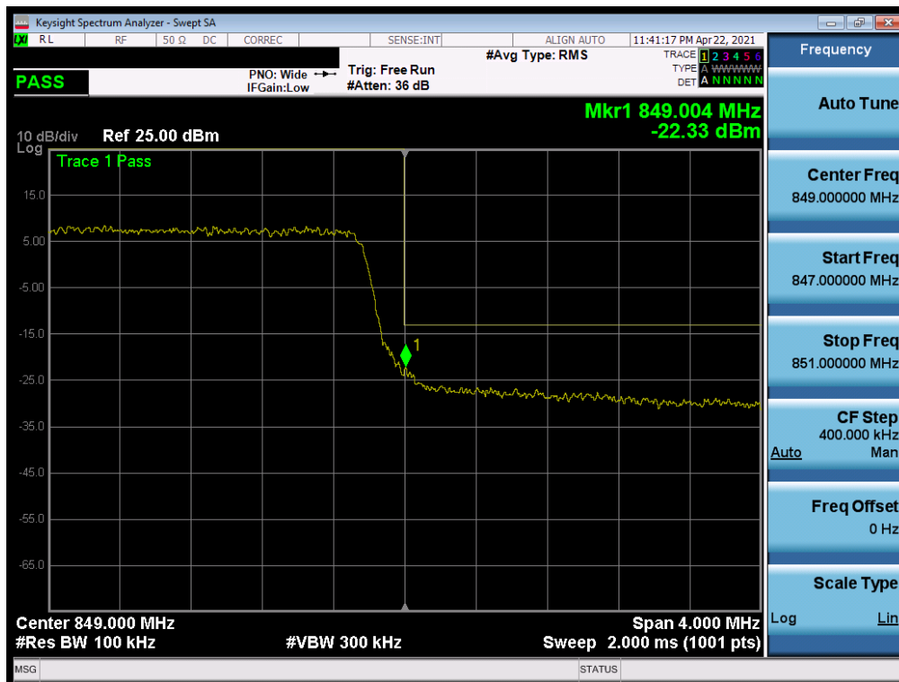
Plot 7-77. Upper Band Edge Plot (LTE Band 26/5 5MHz QPSK – Full RB)
