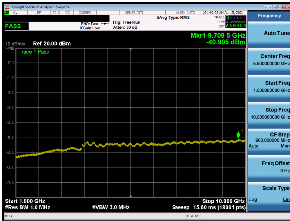
Plot 7-65. Conducted Spurious Plot (CDMA Ch. 1013)
