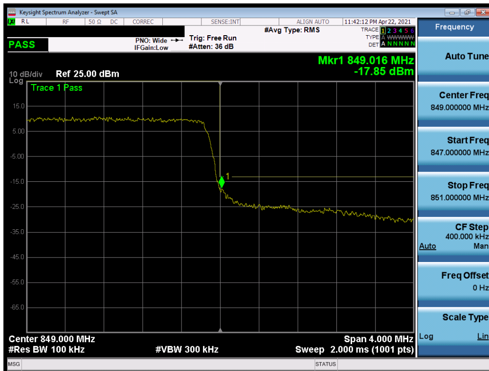
Plot 7-79. Upper Band Edge Plot (LTE Band 26/5 3MHz QPSK – Full RB)
