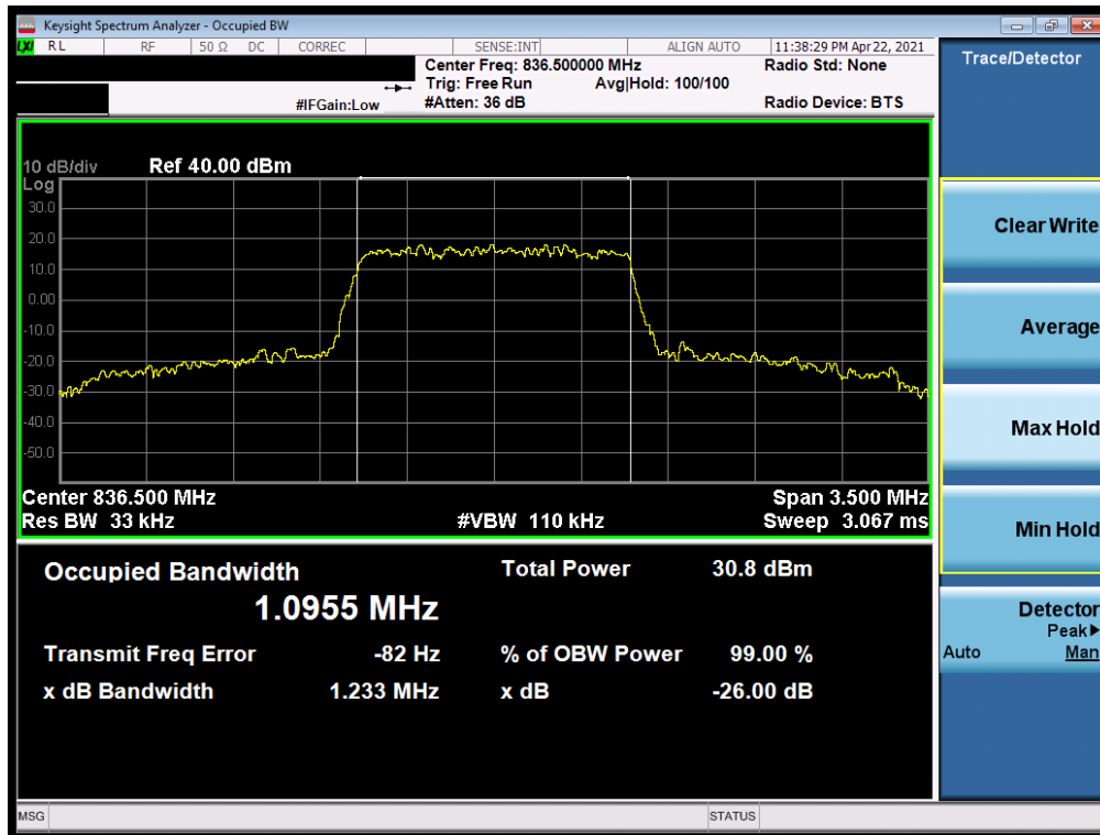
Plot 7-9. Occupied Bandwidth Plot (LTE Band 26/5 1.4MHz QPSK Full RB)
