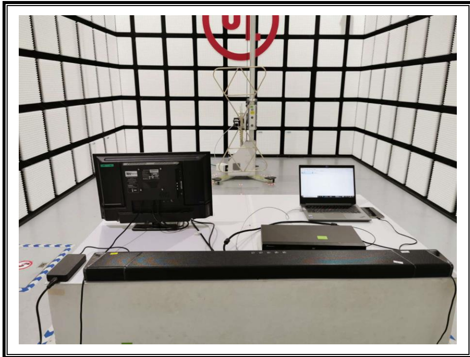
RADIATED RF MEASUREMENT SETUP (Below 30MHz)
