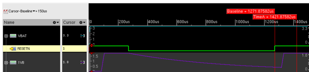
Figure 5: Typical Timing Diagram for Reset Sequence
