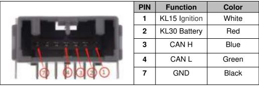
One cable with connectors for connecting the camera unit to the electronic control unit.
