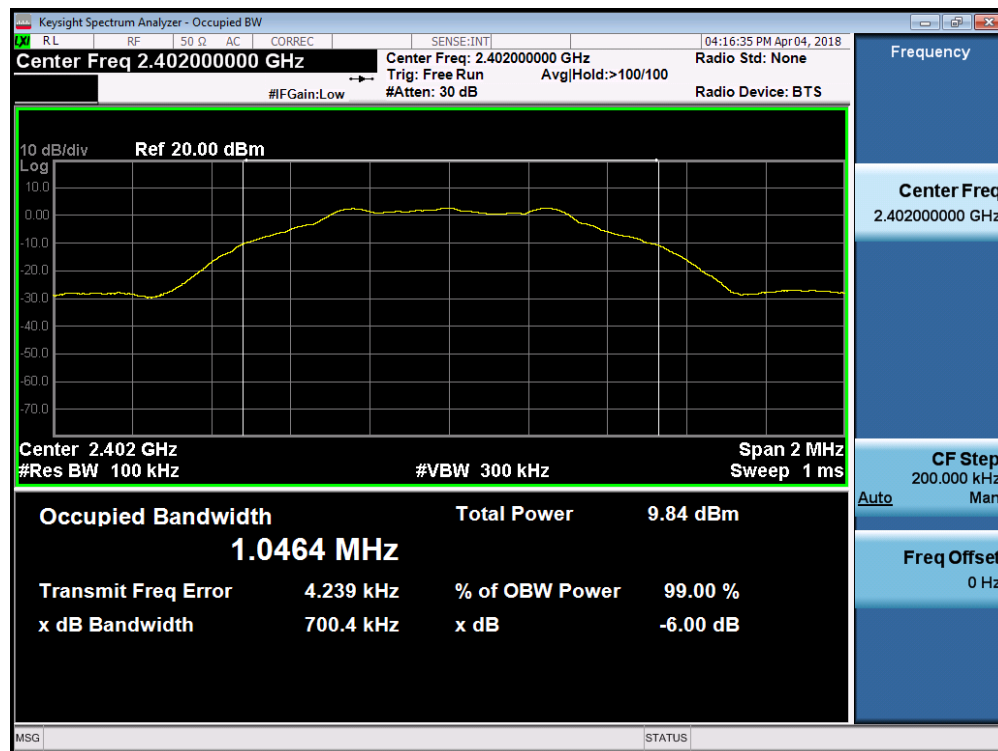
Plot 7-1. 6dB Bandwidth Plot (Bluetooth (LE), Ch. 0)
