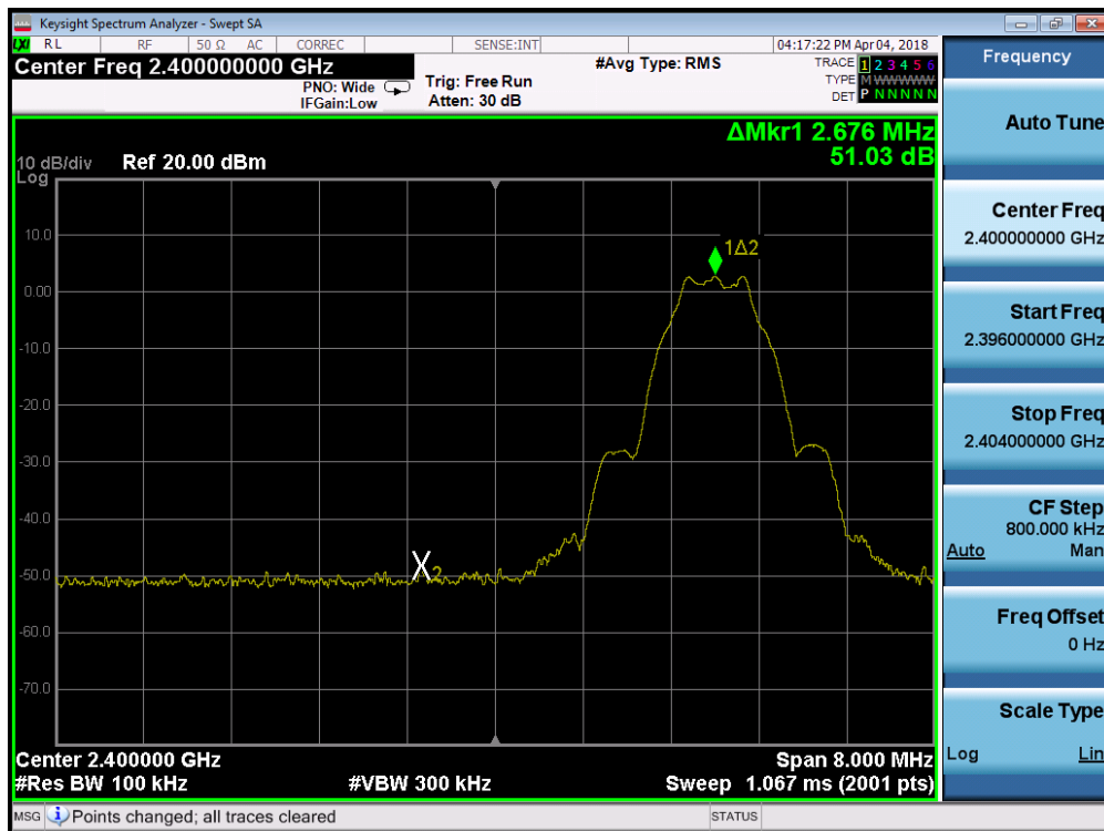
Plot 7-10. Band Edge Plot (Bluetooth (LE), Ch. 0)
