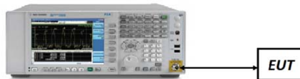
Figure 7-1. Test Instrument & Measurement Setup
