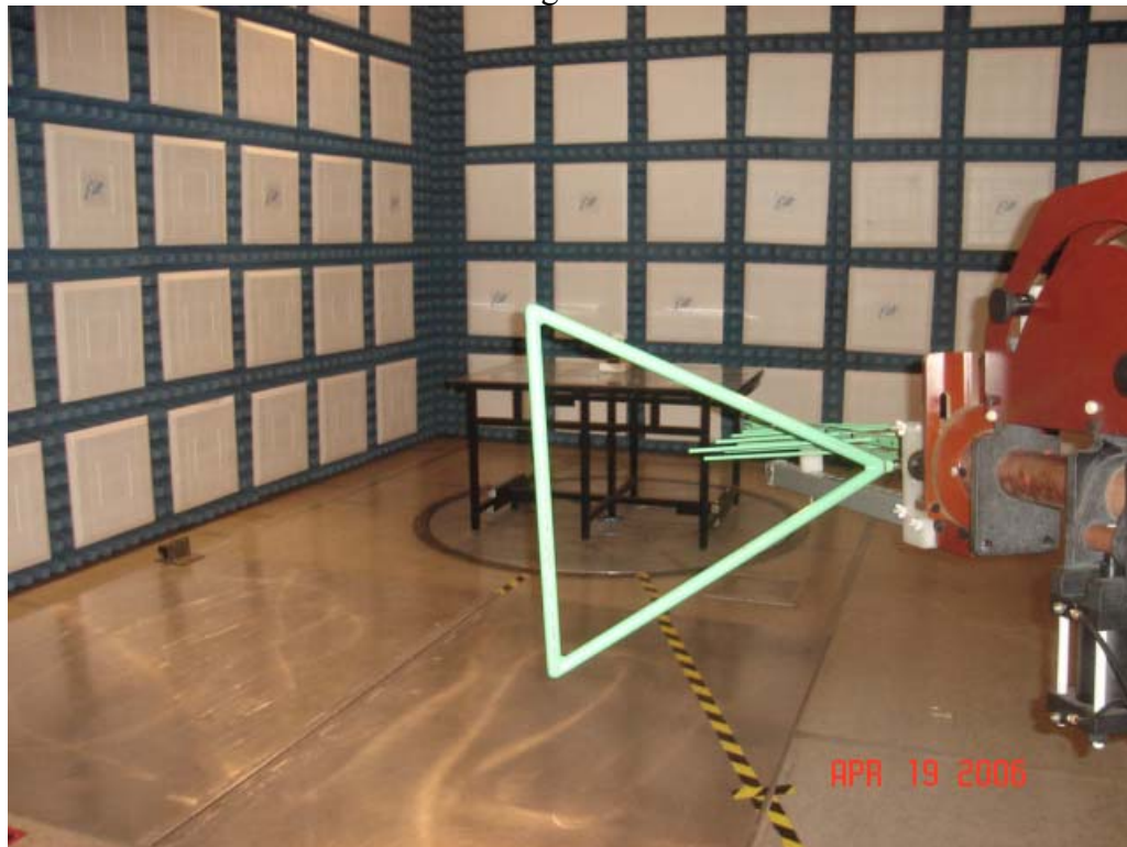
Test Set-up for Radiated Emissions – Horizontal Polarization
