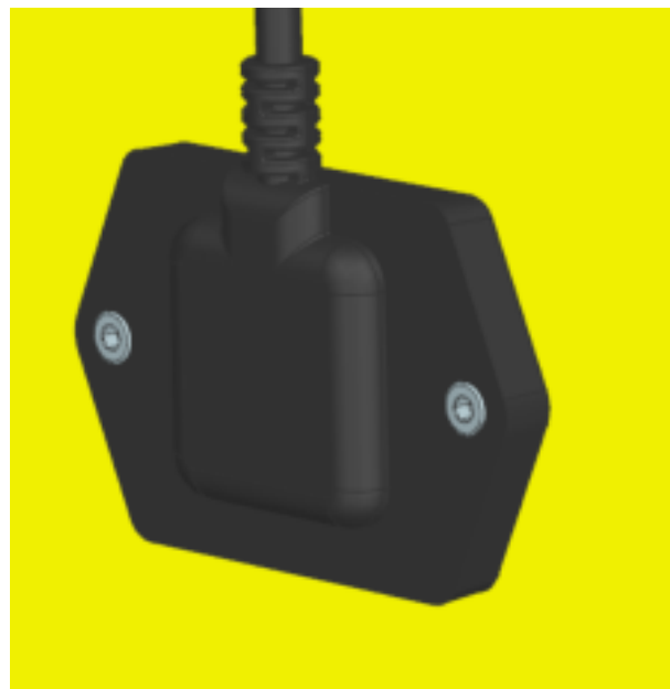
Figure 5-6: RFID Reader top-side mounting illustration
