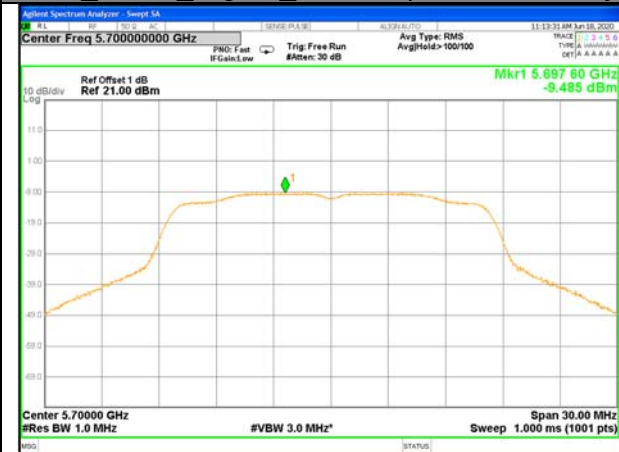
W56_11n20_Middle_Power Spectrum Density
