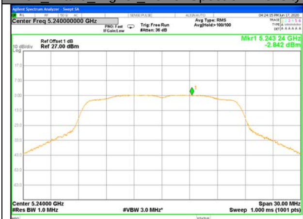
W52_11n20_Middle_Power Spectrum Density
