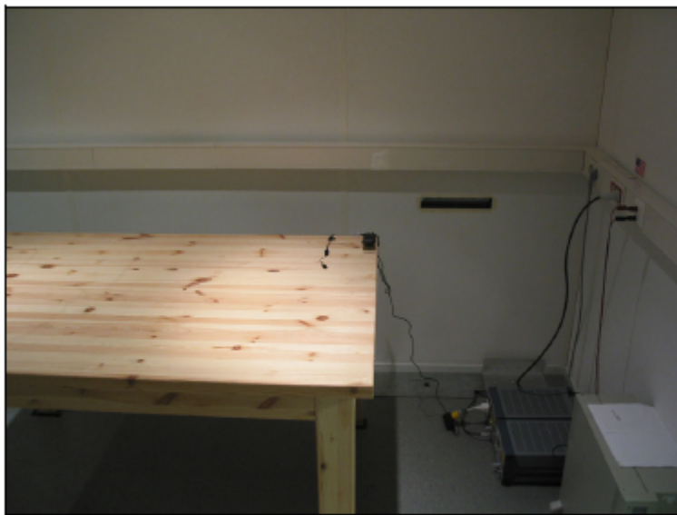
Picture 3 AC conducted emission measurement setup.
