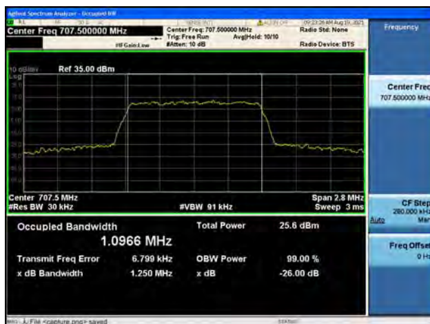
Band12 / 1.4MHz / Mid CH / 16QAM
