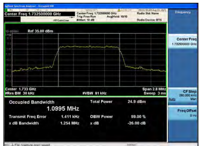
Band4 / 1.4MHz / Mid CH / 64QAM
