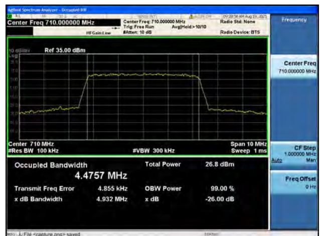
Band17 / 5MHz / Mid CH / 64QAM
