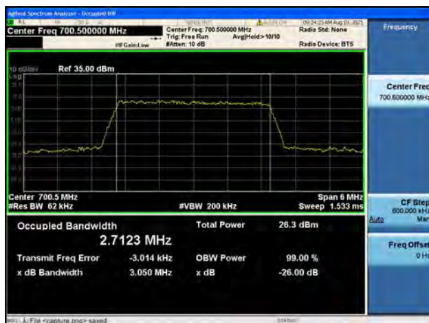
Band12 / 3MHz / Low CH / 16QAM
