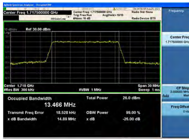
Band66 / 15MHz / Mid CH / 16QAM
