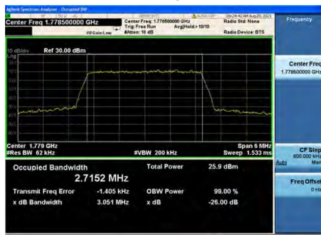
Band66 / 3MHz / High CH / 16QAM
