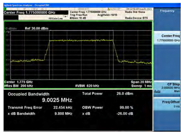
Band66 / 10MHz / High CH / 64QAM
