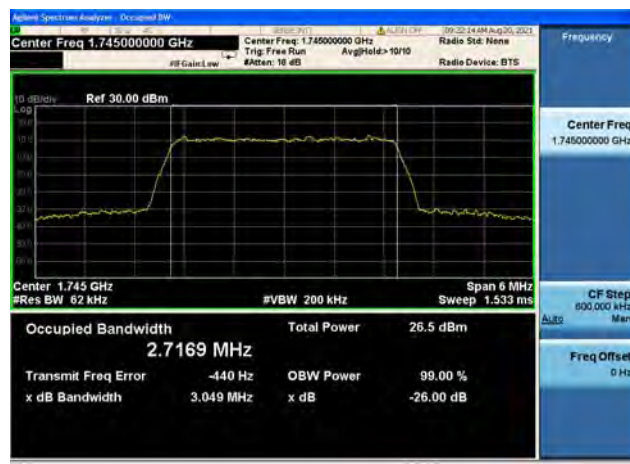
Band66 / 3MHz / Mid CH / 64QAM
