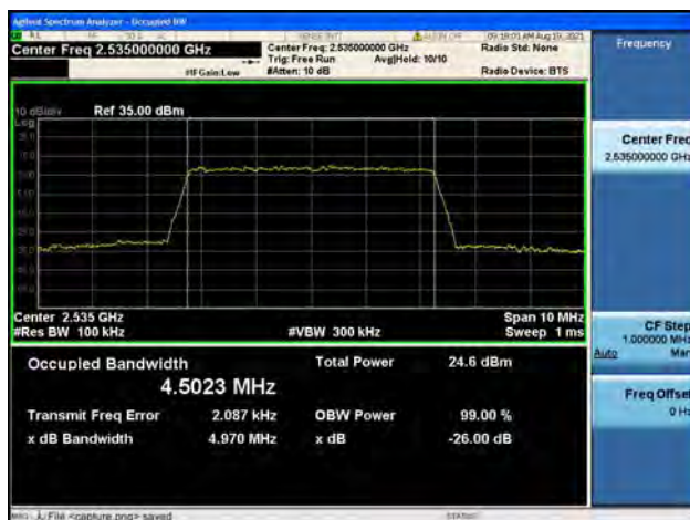
Band7 / 5MHz / Mid CH / 16QAM
