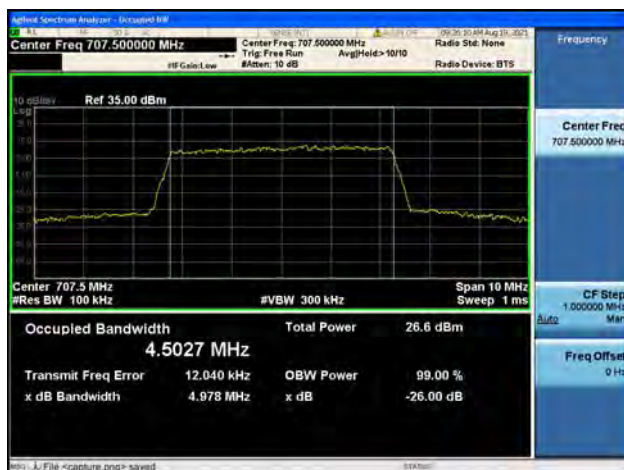
Band12 / 5MHz / Mid CH / 16QAM
