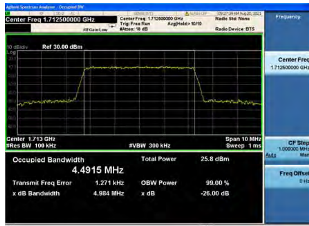
Band66 / 5MHz / Mid CH / 16QAM
