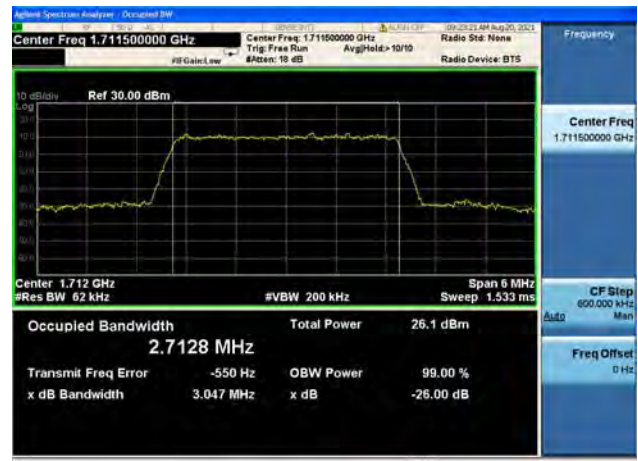
Band66 / 3MHz / Low CH / 64QAM
