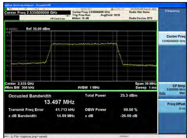
Band7 / 15MHz / Mid CH / 64QAM
