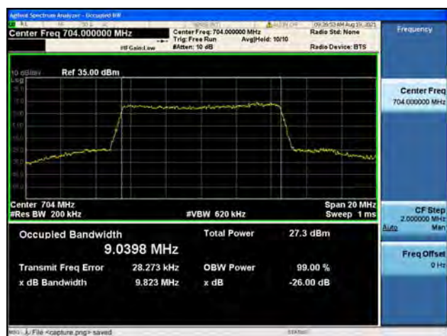
Band12 / 10MHz / Low CH / 64QAM
