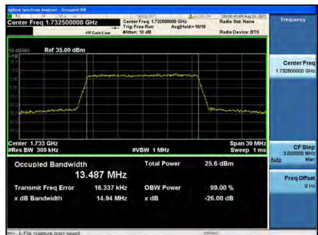
Band4 / 15MHz / Mid CH / 64QAM
