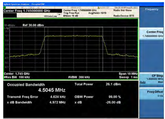
Band66 / 5MHz / Mid CH / 64QAM
