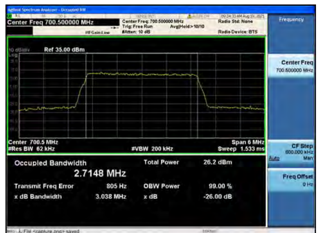
Band12 / 3MHz / Low CH / 64QAM
