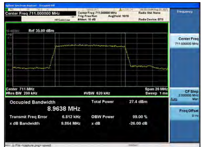
Band17 / 10MHz / High CH / 64QAM
