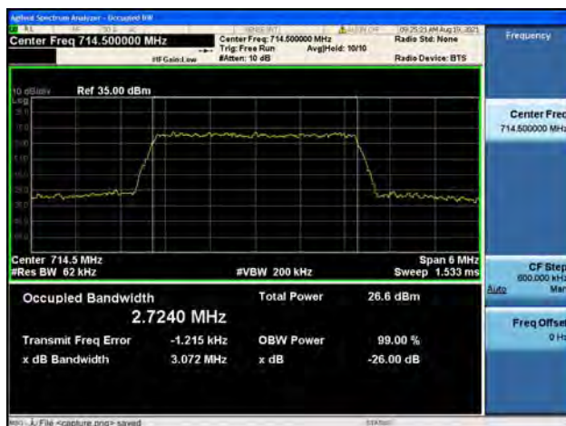
Band12 / 3MHz / High CH / 16QAM
