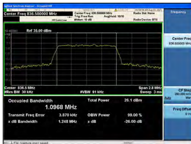
Band5 / 1.4MHz / Mid CH / 16QAM
