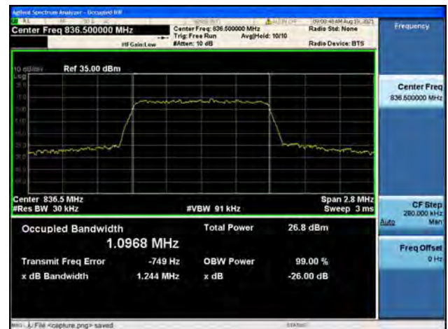
Band5 / 1.4MHz / Mid CH / 64QAM
