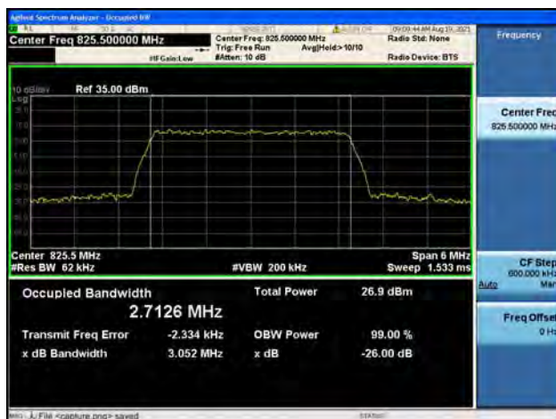
Band5 / 3MHz / Low CH / 16QAM
