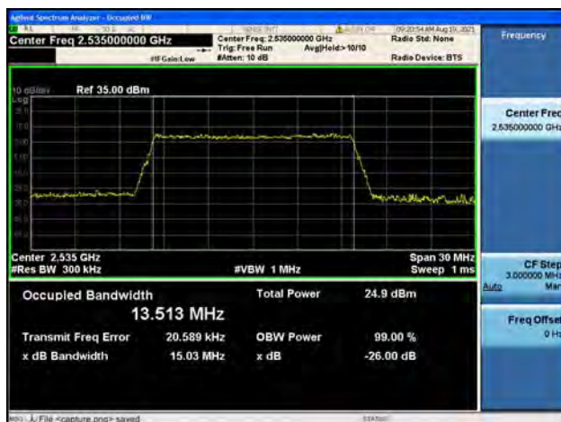
Band7 / 15MHz / Mid CH / 16QAM
