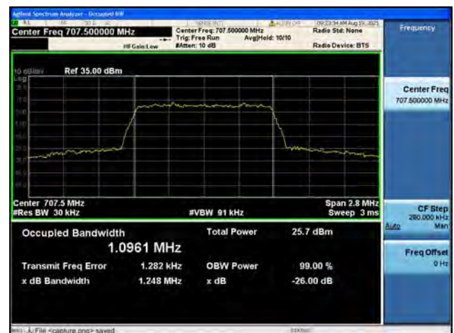
Band12 / 1.4MHz / Mid CH / 64QAM
