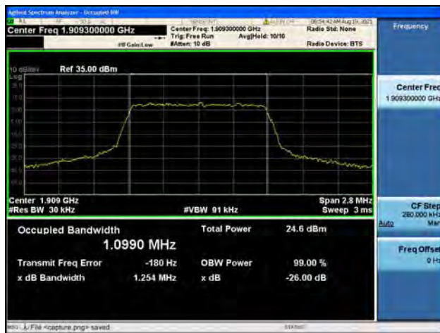
Band2 / 3MHz / Low CH / 16QAM
