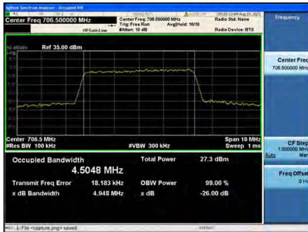
Band17 / 5MHz / Low CH / 64QAM
