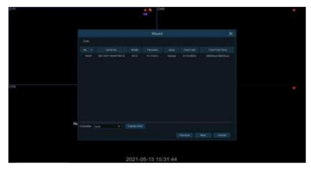
When the hard disk is first installed on the NVR, it needs to be formatted. Select the hard disk and then click the "FormatHDD" icon to format the hard disk.
