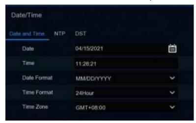
Click on the NTP page to set the time synchronization function. Check the "NTP" box, select an NTP server, and enable the NTP function. When this function is enabled, the device will automatically synchronize the date and time of the selected time server. To ensure the normal use of this function, it is necessary to ensure that the device is connected to the network.
