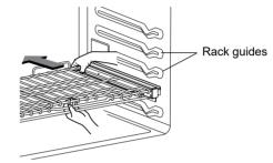
3 Once the rack is secured in the back, pull the entire rack forward until the rack locks into place.
