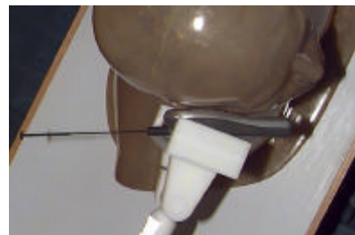
Fig. 16 Head SAR Test Setup
