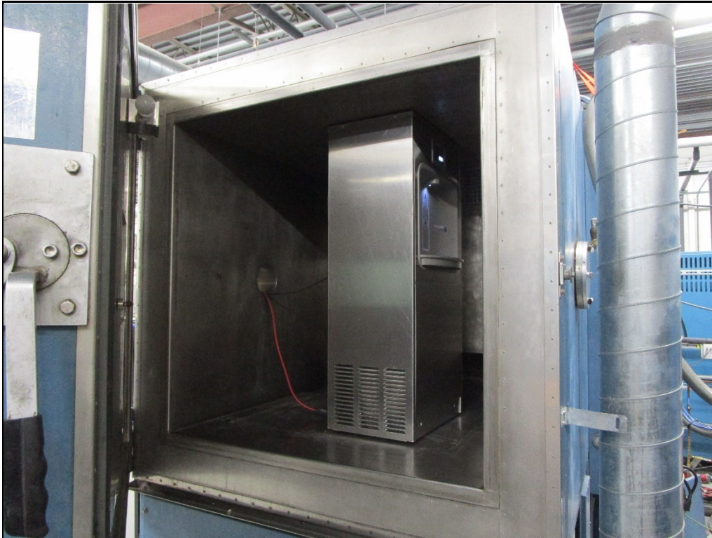
Test Setup for Frequency Stability
