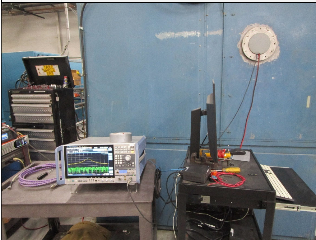
Test Setup for Frequency Stability
