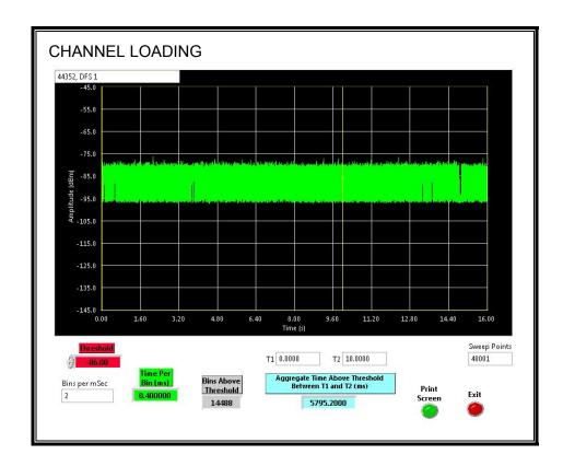
The level of traffic loading on the channel by the EUT is 57.952%.
