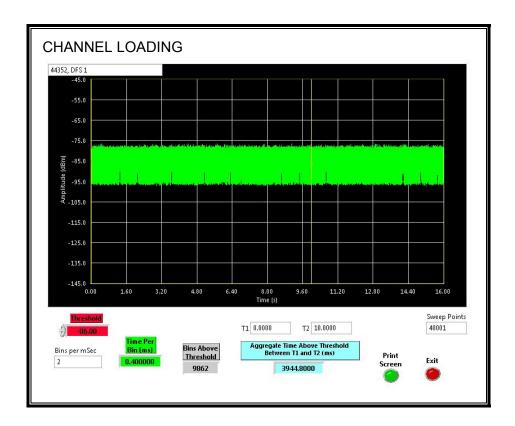
The level of traffic loading on the channel by the EUT is 39.448%.
