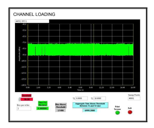
The level of traffic loading on the channel by the EUT is 69.992%.
