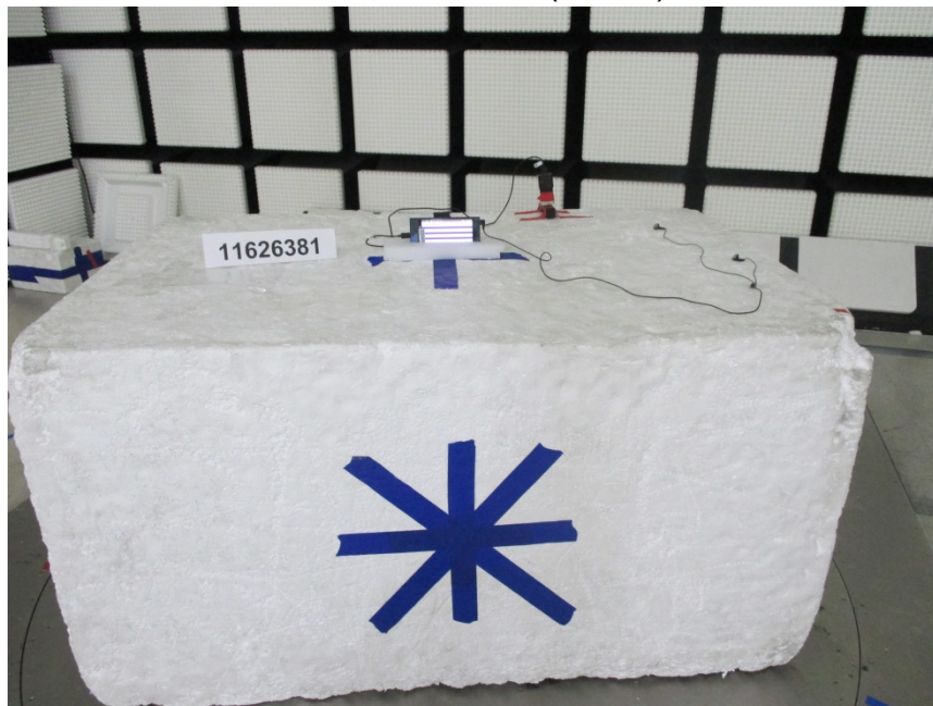
RADIATED EMISSIONS ABOVE 30 MHz (FRONT)
