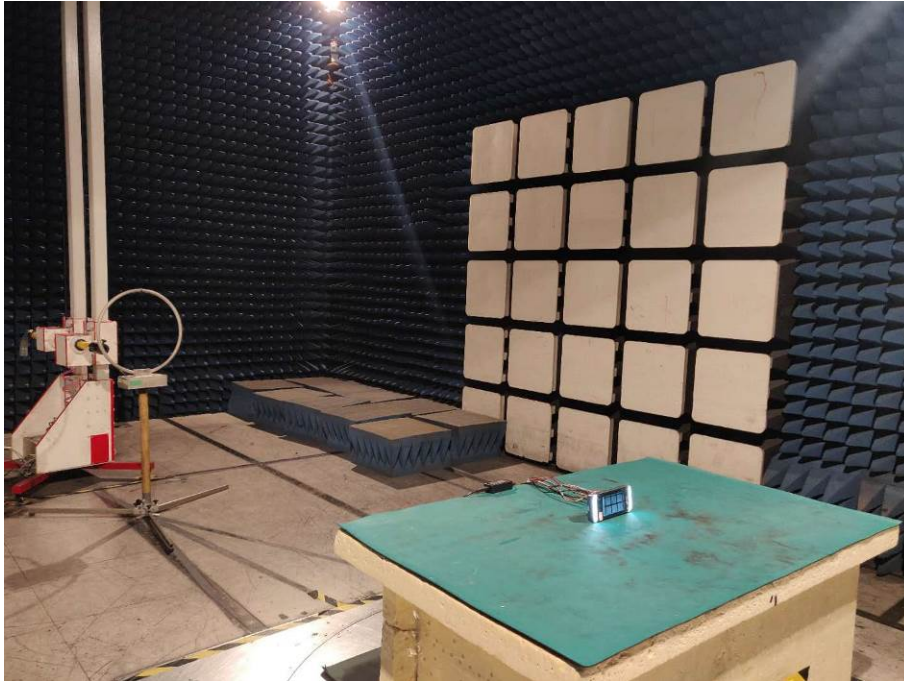
Spurious Emission Test Setup (Below 30MHz)
