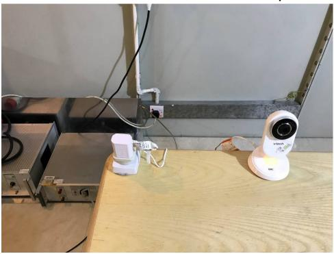
Radiated Emissions (30MHz-1GHz) Test Setup
