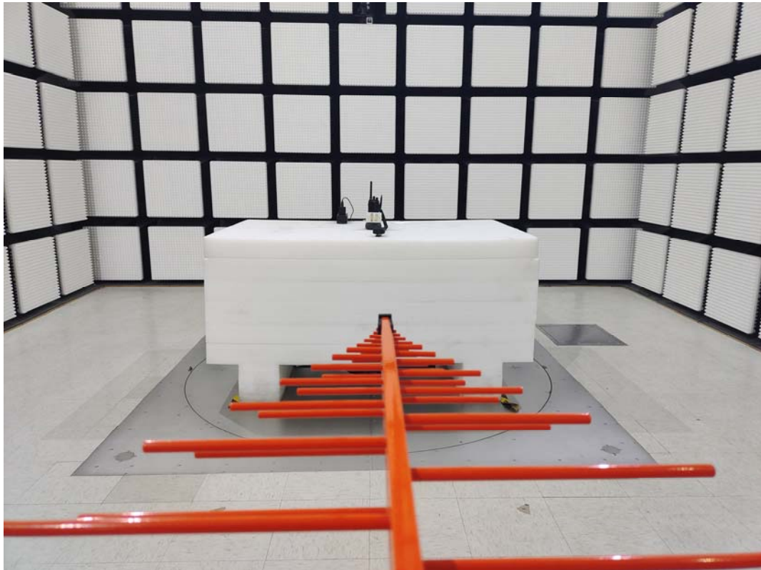
Radiated Emission Below 1GHz View
