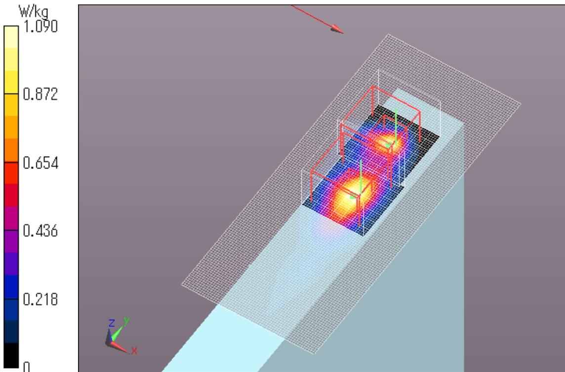
**WLAN 11a 6Mbps Main Ant Edge4 5560MHz**
