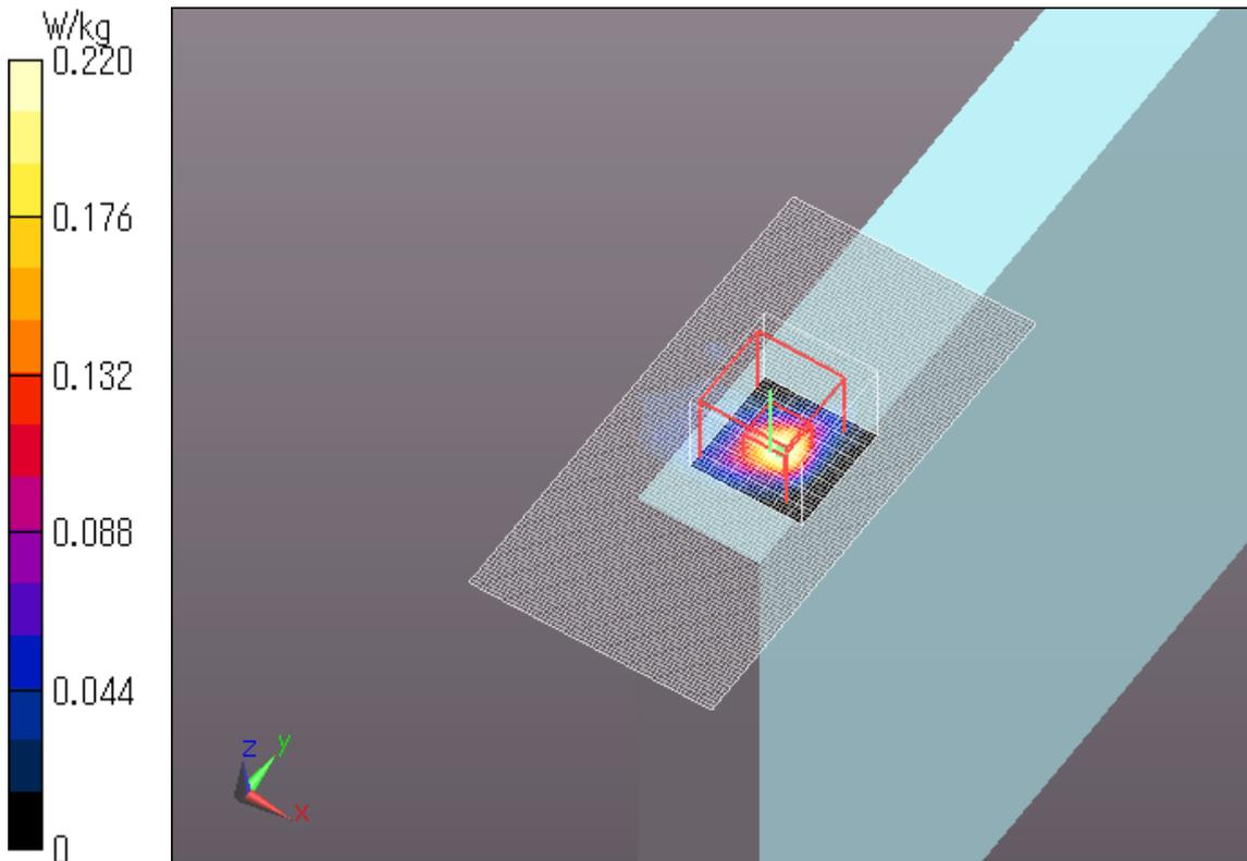
**WLAN 11a 6Mbps Main Ant Edge4 5280MHz**
