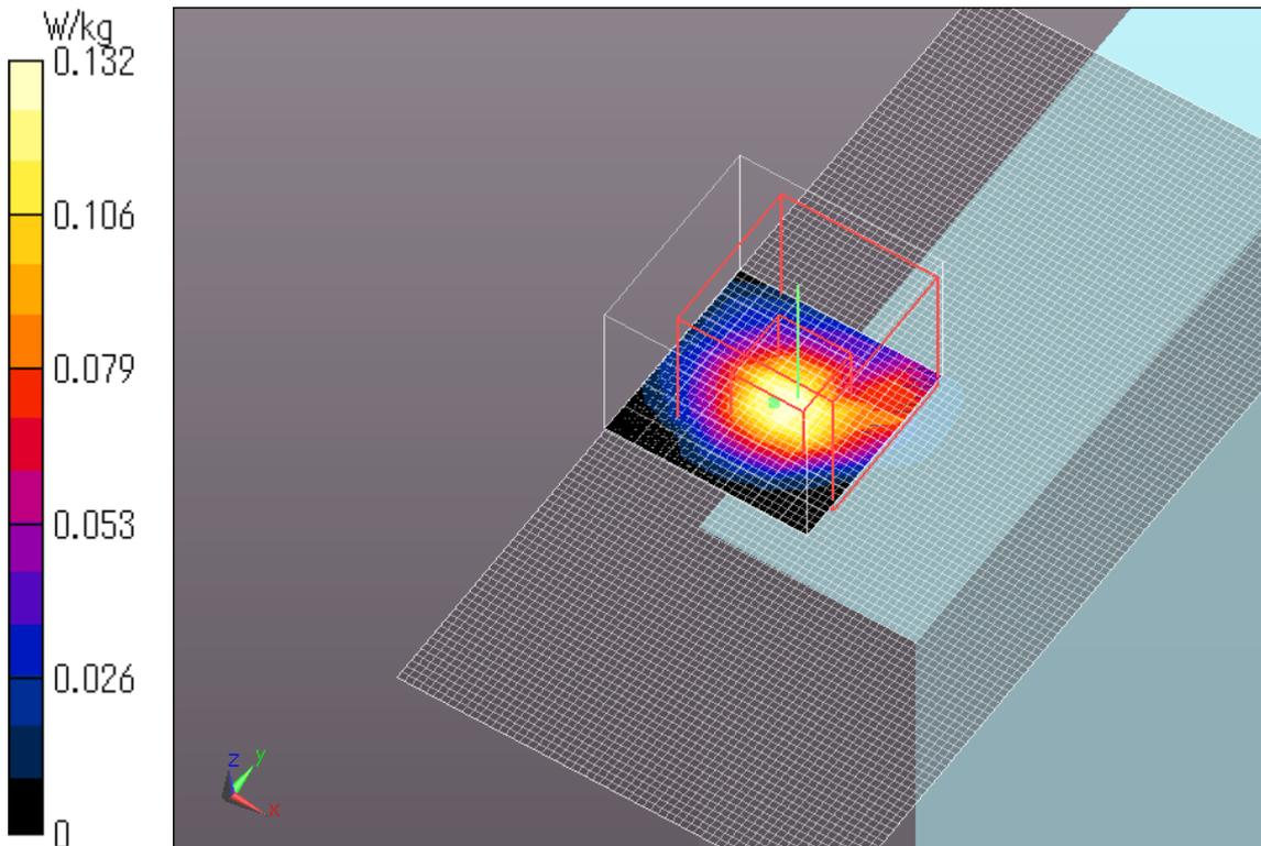
**WLAN 11a 6Mbps Main Ant Edge4 5500MHz**
