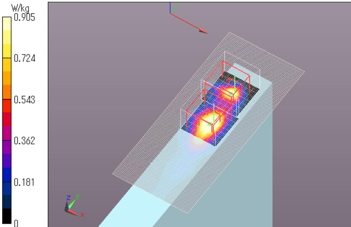
**WLAN 11a 6Mbps Main Ant Edge4 5700MHz**
