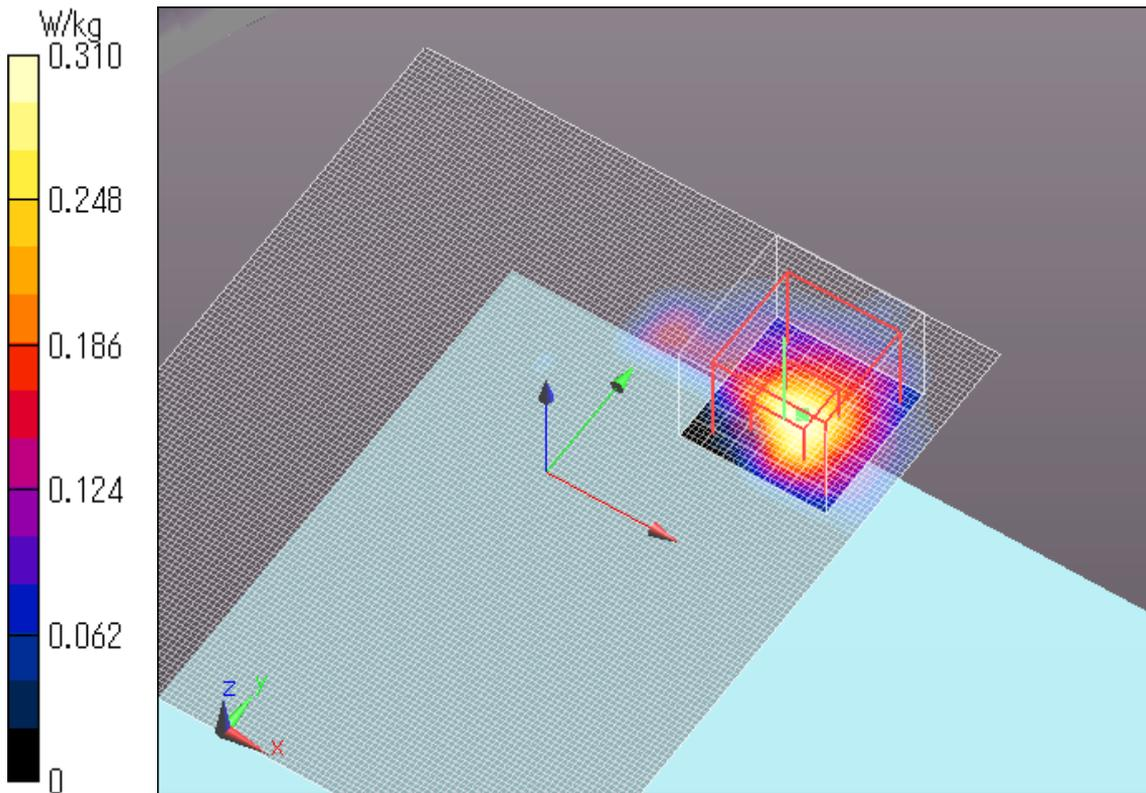
**WLAN 11a 6Mbps Main Ant Edge1 5785MHz**
