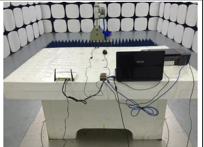
Radiated Emissions Test Setup Above 1GHz
