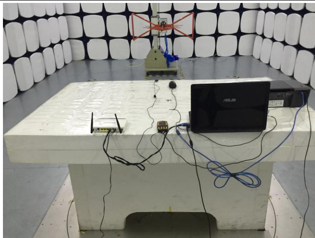
Radiated Emissions Test Setup Below 1GHz
