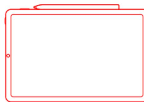
Please attach the stylus body horizontally to the centre of the long side of the tablet (as shown in the figure), perform Bluetooth pairing and start charging.
