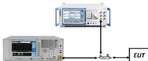
Figure 7-3. Test Instrument & Measurement Setup
