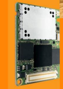
Siemens presents its MC75, making it the first vendor to introduce a GSM/GPRS module with integrated EDGE technology. This module handles highly data-intensive multimedia applications – such as downloading and streaming of audio and video data, transmission of digital photos and instant messaging services – with exceptional speed and reliability. With Quad-Band capability, the MC75 can be used in all the existing GSM networks in America, Europe and Asia, guaranteeing seamless communication.
